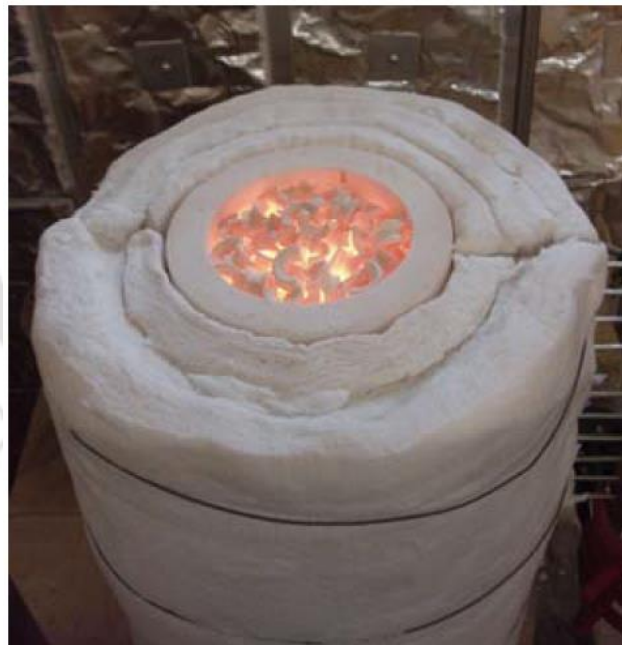
Figure 1.1: Combustion in porous media (a) Schematic of a basic configuration of porous burner (b) Heated surface of volumetric porous burner
