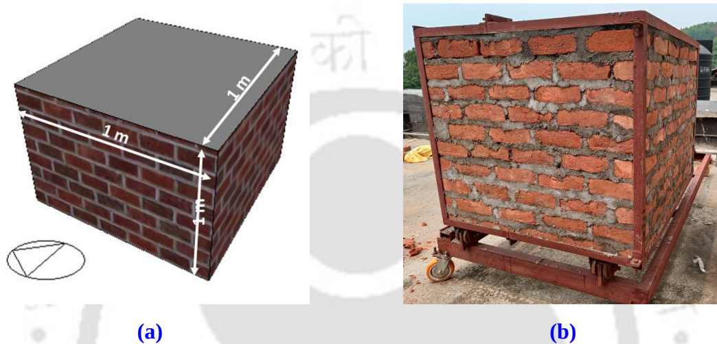
Fig. 5.3 Building model for validation, (a) Numerical model, (b) Experimental set-up
