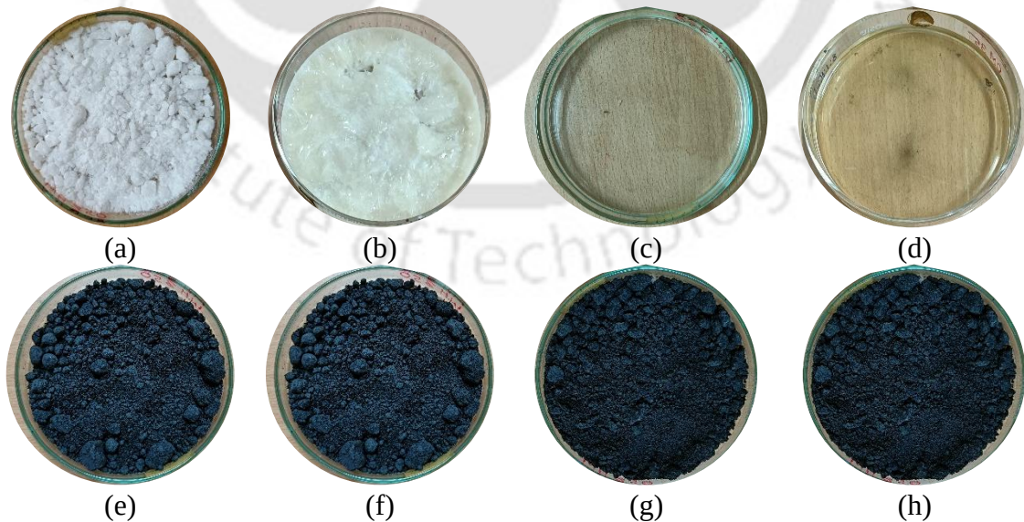
Fig. 3.16 Images of PCMs before and after thermal cycling test, (a) OM 35_0 (solid), (b) OM35_200 (solid), (c) OM 35_0 (liquid), (d) OM 35_200 (liquid), (e) WH-PCM_0, (f) WH-PCM_200, (g) T 0 -SWY PCM_0, (h) T 0 -SWY PCM_200
