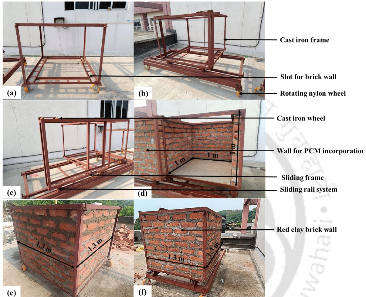
Fig. 4.7 Development of prototype buildings (a) Frame for reference cubicle, (b) Frame for PCM cubicle, (c) Sliding rail provision for PCM cubicle, (d) Interior of the developed PCM cubicle, (e) Reference cubicle outer view, (f) PCM cubicle outer view
