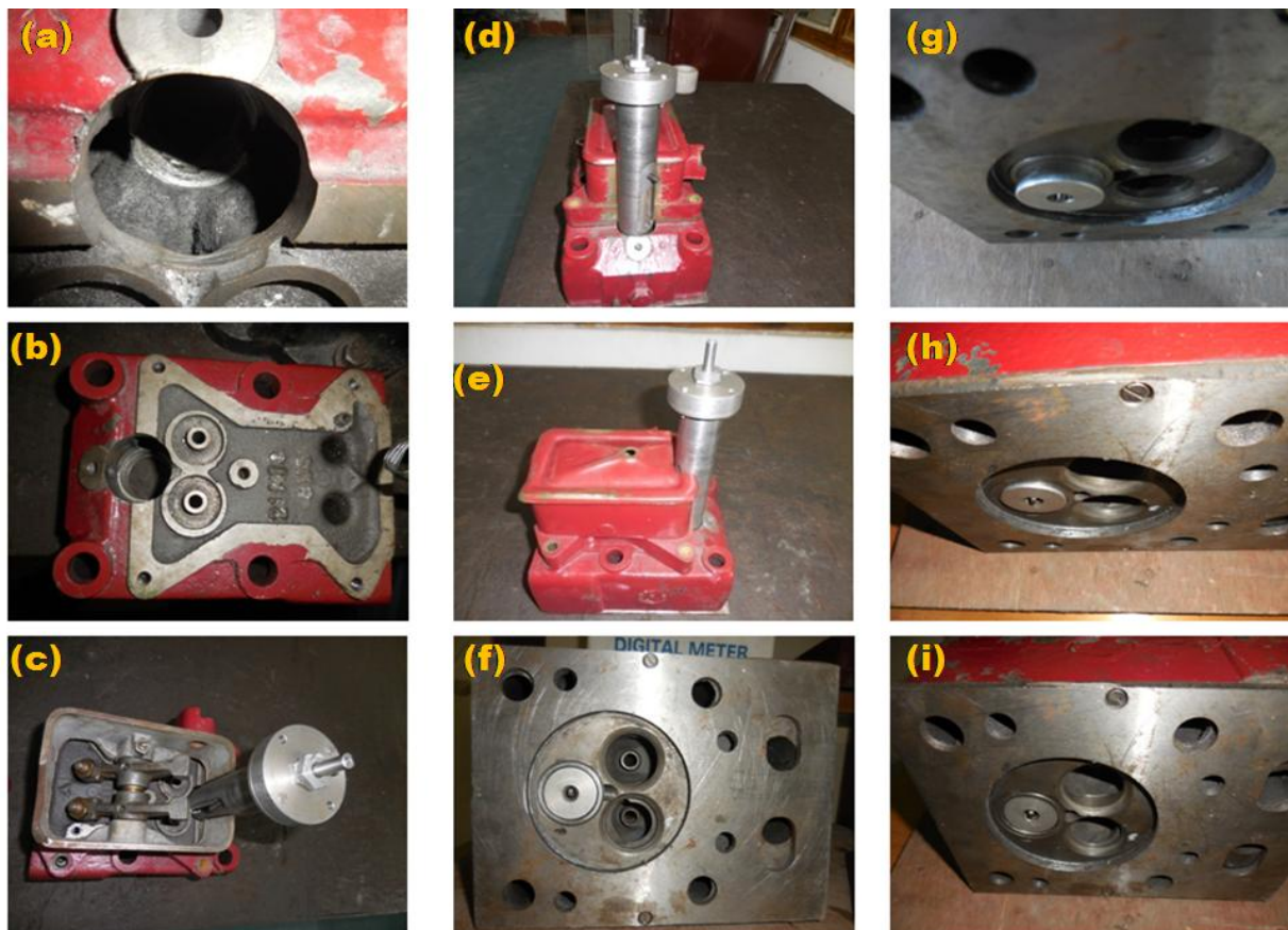
Fig. 4.17 The procedure of mounting novel VCR mechanism on the engine head following procedure (a) The provision made for mounting VCR mechanism; (b) the drill of 31.8 mm diameter with thread inside over 40 mm depth; (c) the novel VCR mechanism fixed over engine ; (d) the assembly of engine head with novel VCR; (e) the space consumed on the convention engine; (f) the inside structure of the engine head occupying suction, exhaust valve and third is secondary piston arranged very precisely; (g) the secondary piston displacement of 5 mm inside combustion chamber;(h) the secondary piston displacement of 2 mm inside combustion chamber;(i) the secondary piston displacement of 0 mm inside combustion chamber.
