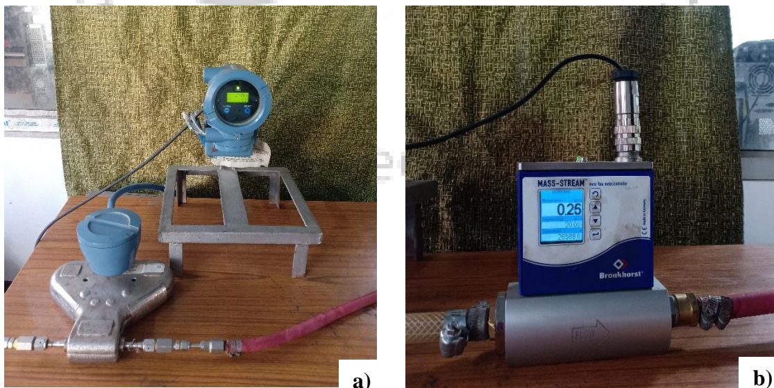
Fig. 3.5: Mass flow meter a) for fuel and b) for air
