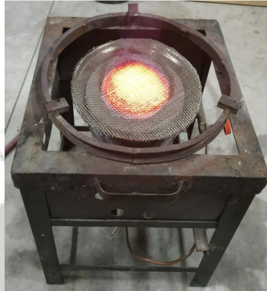
Fig. 5.1: Self-aspirated PRB (5 – 7 kW) developed by Muthukumar et al. (2020)
