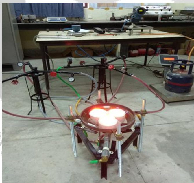
Fig. 3.13: Photographic view of the CPRB under stable operation
