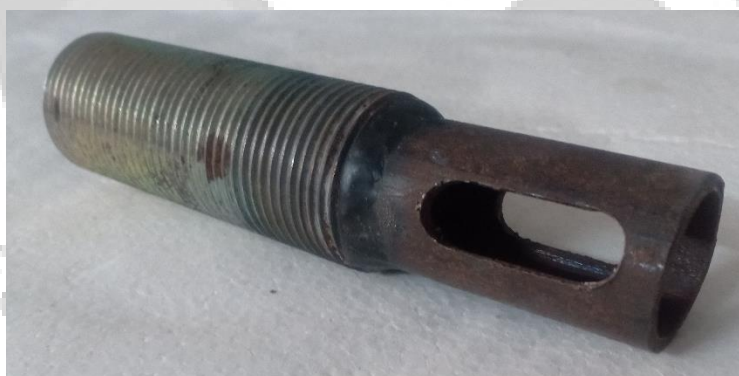
Fig. 4.2: Typical mixing tube used in self-aspirated PRB cookstoves
