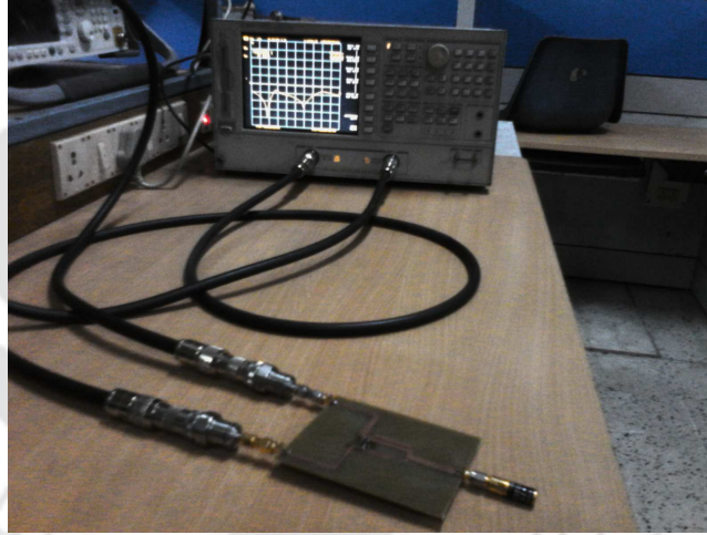
Figure 5.14: Setup for isolation measurement.
