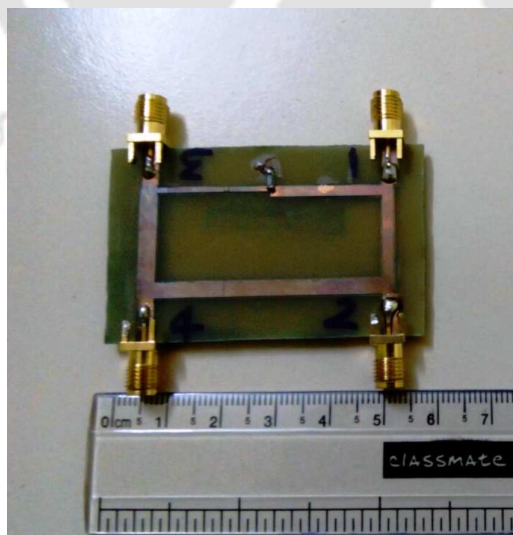
Figure 3.35: Fabricated prototype of power divider for power division ratio k^2 = 2 .
