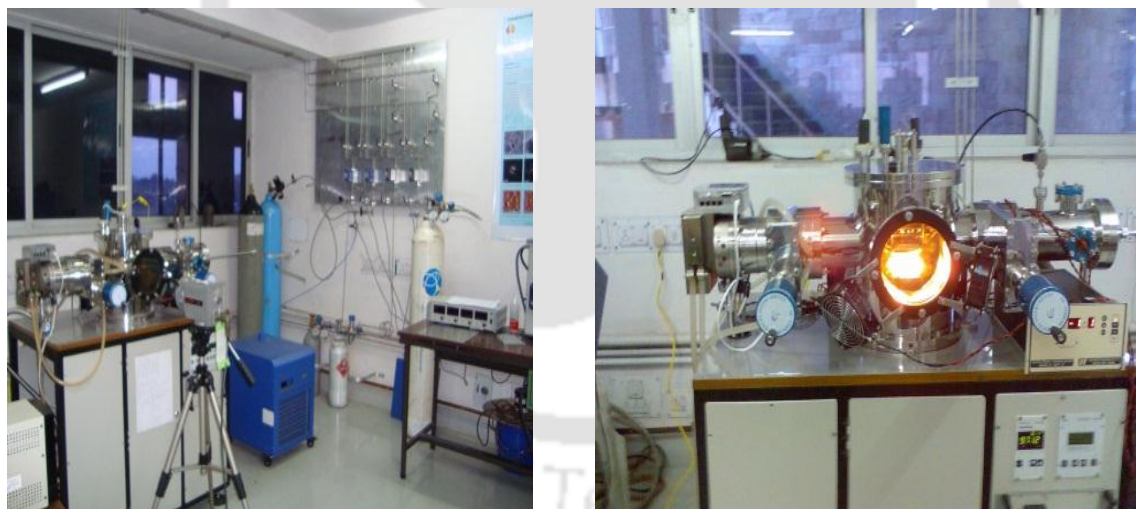
Figure 2.2: The fabricated HWCVD system with gas manifold in the laboratory (left). HWCVD system during films deposition (right).
