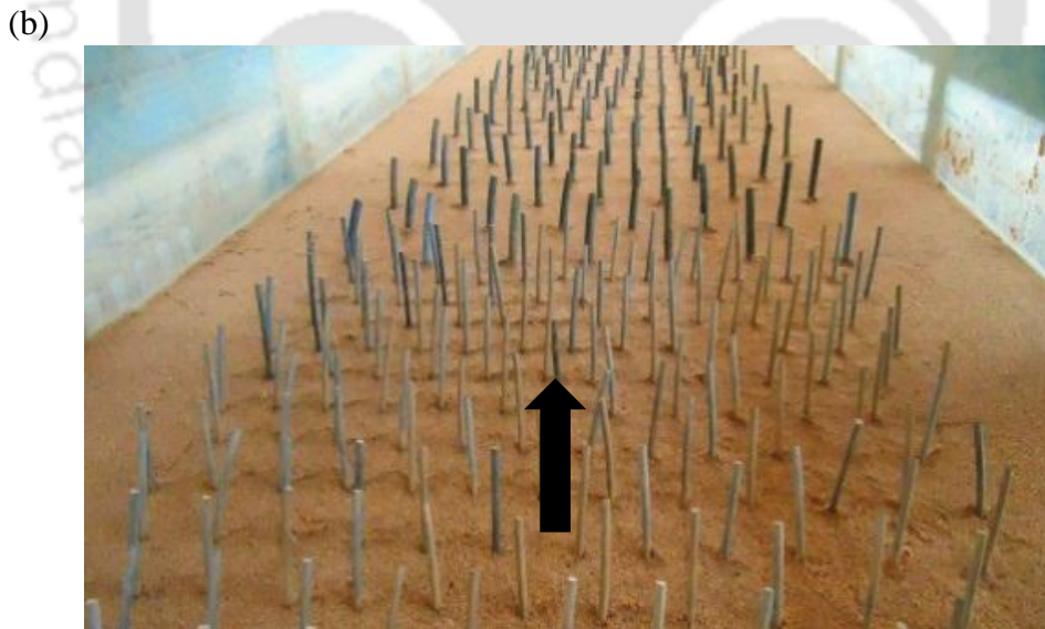
Figure 2.15 Mixed vegetation pattern of placing 5 mm diameter upstream and 10 mm downstream
