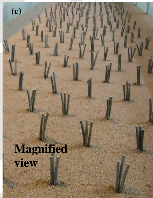
Figure 2.16 Experimental set-up (a) Test section with measurement locations (b) Photograph taken after placing of vegetation patches (c) Magnified view of vegetation patches
