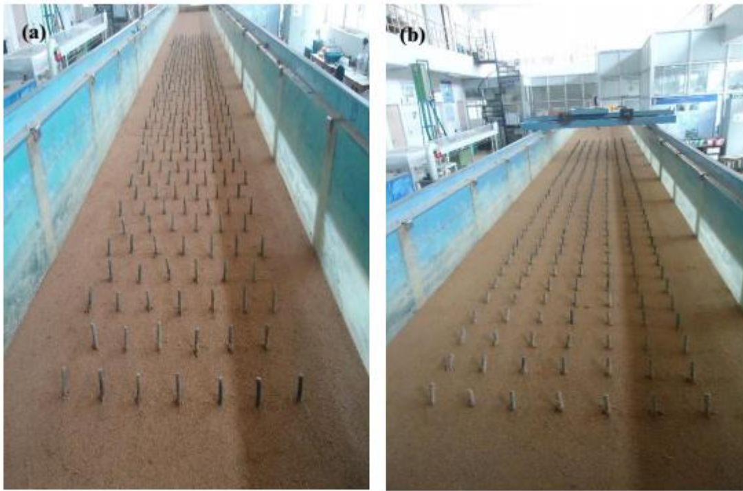
Figure 2.13 Photographs showing the placing of cylinder stems as artificial vegetation (a) staggered (b) uniform
