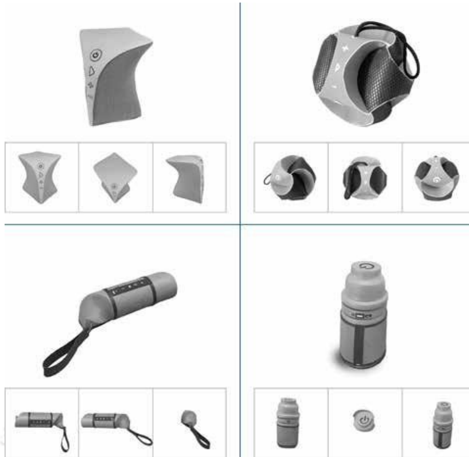
Figure. 4.3: 3D CAD renders of Bluetooth Speaker Concept Sketches
