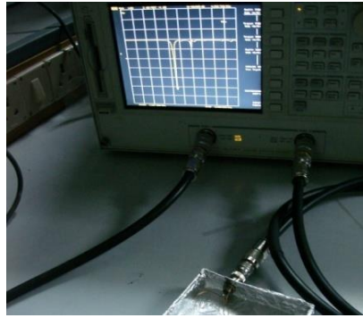
Figure 7. 4: The set up showing network analyser for testing the device.
