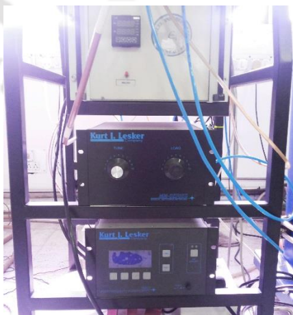
Figure 7. 20: The RF power source used for testing the device.
