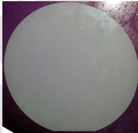
Figure 6. 12: Picture of an LN ( \text{LiNbO}_3 ) wafer after cleaning.
