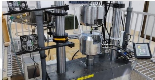
Fig. 2.52 Test set-up for tensile test
