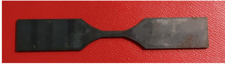
Fig. 2.51 Fabricated coupon specimen
