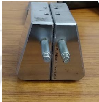
Fig. 2.49 Wedge type flat grips used for flat specimens
