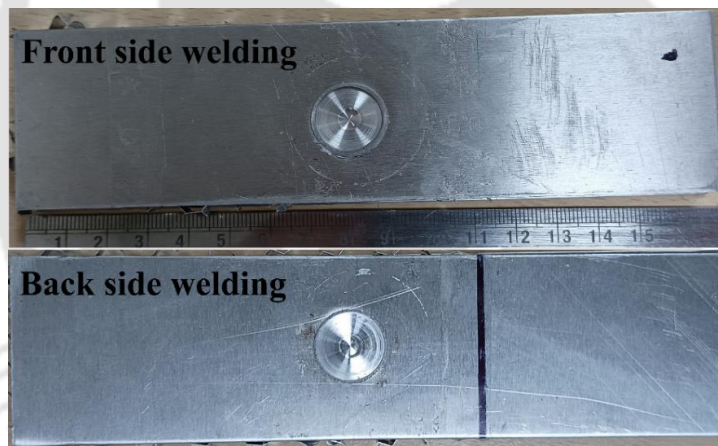
Figure 7.2 Fabricated peel specimen by FSSW_D process
