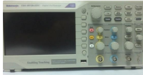
[Specification: Make (Tektronix); Model (TDS2001C/TBS1072B-EDU); Description: Bandwidth : 50/70 MHz; Channel : 2 Analog Channels; Sampling Rate : 500 MS/s/ 1 GS/s; Record Length: 2.5k points at all-time bases]
