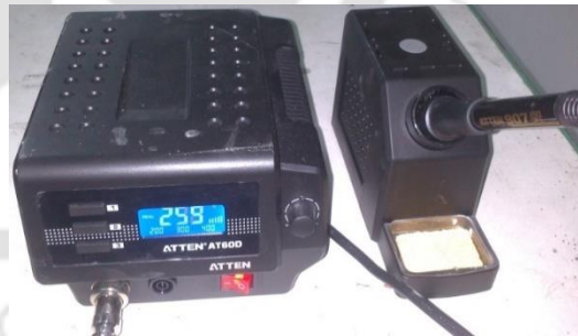
[Specification: Make (RS Components & Controls (India) Ltd; Model (AT60D, 7998939), 220 V, AC 60 W]
