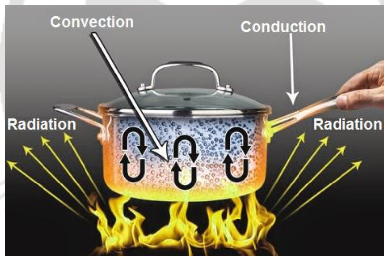
Fig. 1.1: Schematic highlighting the modes of heat transfer ( https://me-mechanicalengineering.com/modes-of-heat-transfer/ )
