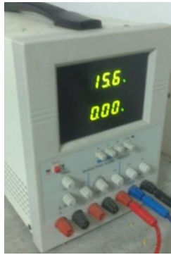
[Specification: Make (ScientiFic India); Model (PSD3304); 30V-2A, 0 to +/- 15V-1A, 5V-5A Multiple Power Supply]
