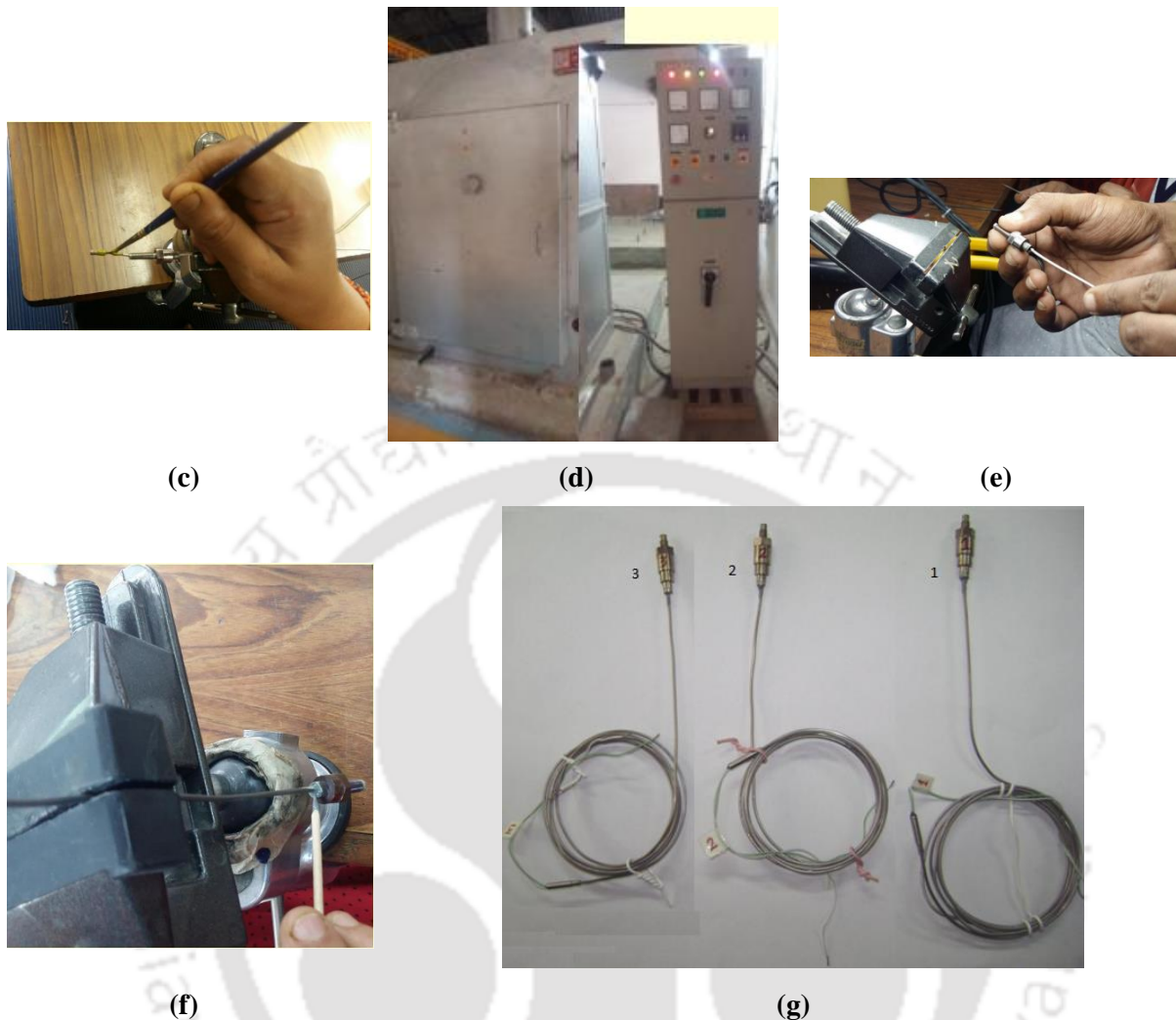
Fig. 9.4: Packaging procedure: (a) barrel for CSJT probe; (b) miniature CSJT probe housed in a barrel; (c) application of ceramic cement for pre-curing of CSJT; (d) furnace for curing CSJT probe; (e) insertion of CSJT in the barrel; (f) application of adhesive for final packaging; (g) packaged sensors for gas turbine engine testing.
