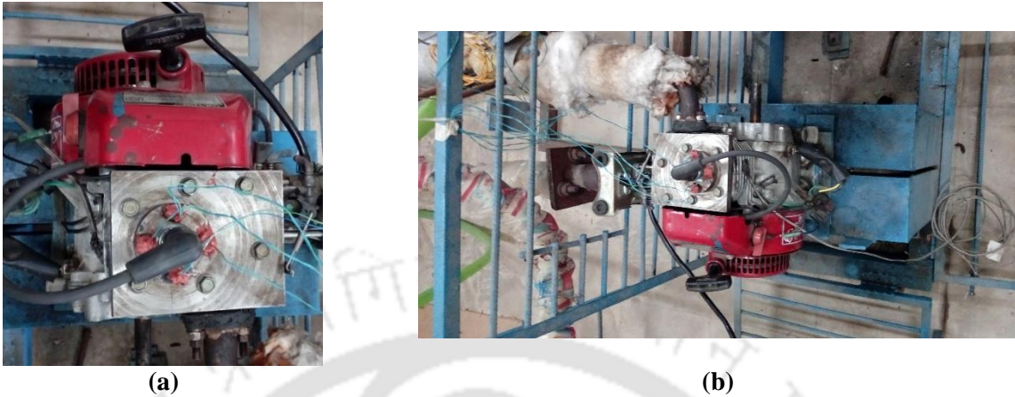
Fig. C.13: Pictorial view of the experimental set-up showing the mounted coaxial thermal sensor
