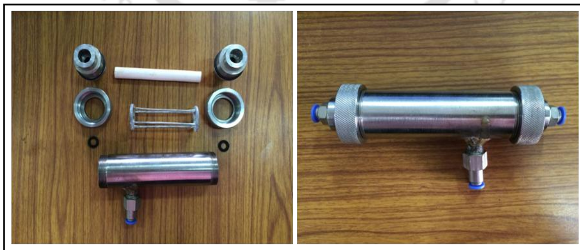
Figure 2.12: Tubular membrane before fixing and after fixing into module
