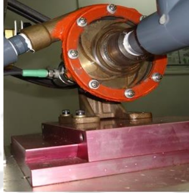
Figure 2.9: Pump mounted on the MFS with a poly-carbonate transparent cover
