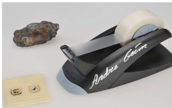
Figure 1.8: Scotch tape method for the mechanical exfoliation of graphene (picture has been taken from the Wikipedia-page of graphene)
