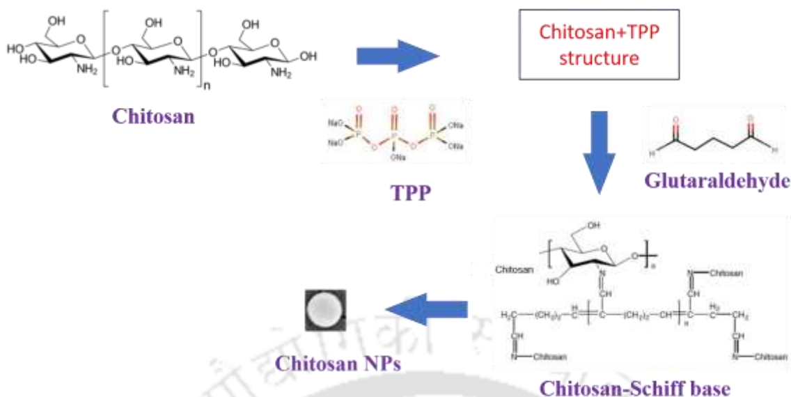
Figure 6.10: Schematic showing the chitosan NPs fabrication strategy.
