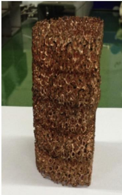
(I) Pictorial view of copper metal foam and copper fin inclusions (Ferekh et al., 2015)
