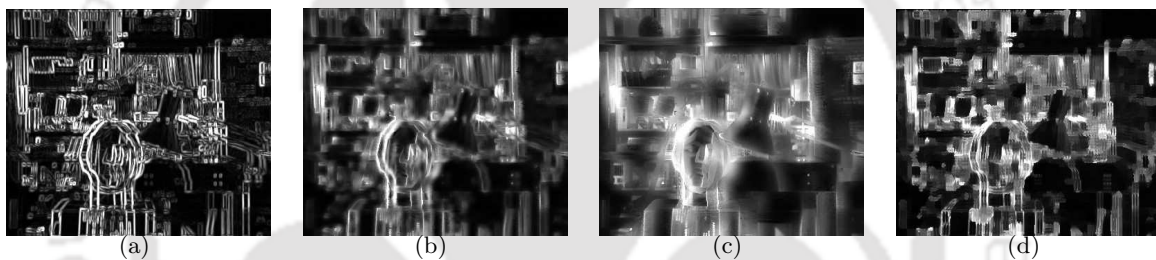
Figure 3.15: Disparity space image filtering. (a) Disparity space image ( d = 1 ); (b) Filtering by guided filter (window size - 3 \times 3 ); (c) Filtering by guided filter (window size - 9 \times 9 ); (d) Filtering by Kuwahara filter (window size - 9 \times 9 ).
