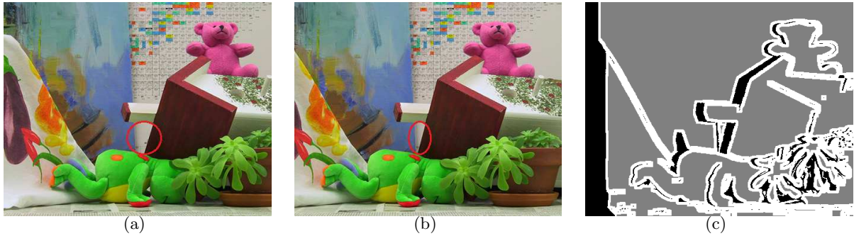
Figure 1.18: Discontinuous regions in stereo images. (a) Left image; (b) Right image; (c) Discontinuous regions [7].
