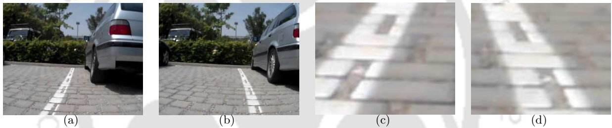
Figure 1.15: Stereo images having perspective distortions. (a) Left image; (b) Right image; (c) Zoomed out region of image (a); (d) Zoomed out region of image (b) [5].
