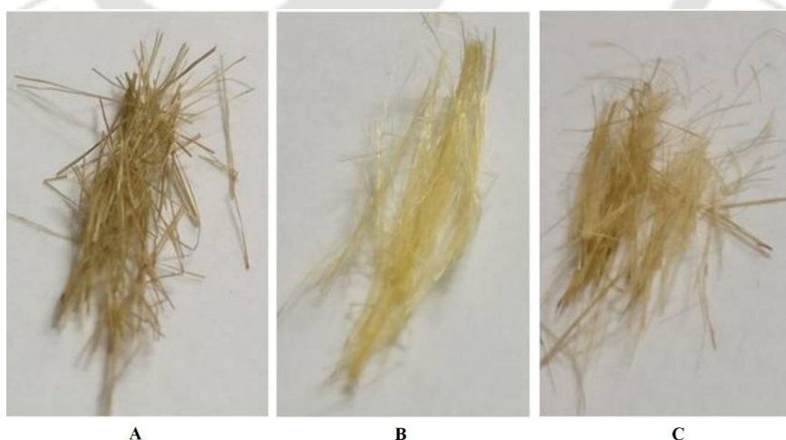
Fig. 6.3 Digital images of (A) CtRGLf untreated jute fibers (negative control), (B) chemical (NaOH) treated jute fibers (positive control) and (C) CtRGLf treated jute fibers.
