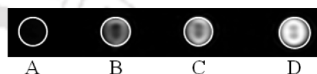
Figure 7. T_1 -weighted phantom MR images of the complex 1 at different concentrations (A = 0.25 mM, B = 0.50 mM, C = 0.70 mM, D = 1.00 mM) at 1.5 T, 25 °C, and pH \sim 7.4.
