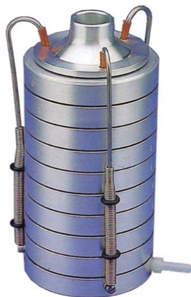
Fig 3.3 Layout of the 8 Stage Non-Viable Cascade Impactor (Series 20-800, Thermo fisher Scientific, Inc.)
