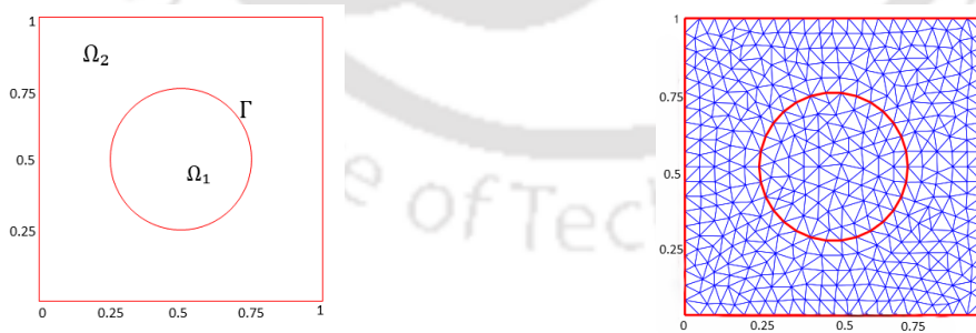
Figure 6.5.1: The domain \Omega with interface \Gamma (left) and a refined mesh (right) at level 6.
