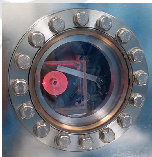
Figure 6.7: Resonator under characterization in ultra high vacuum chamber and LDV measurement
