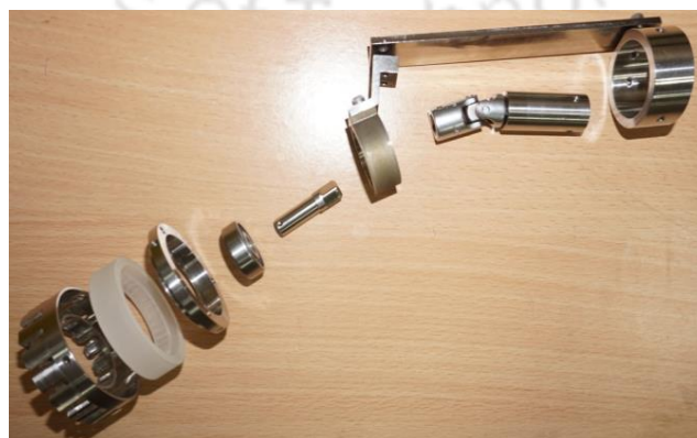
Figure 8.2: Realized components and subassemblies of glancing mechanism
