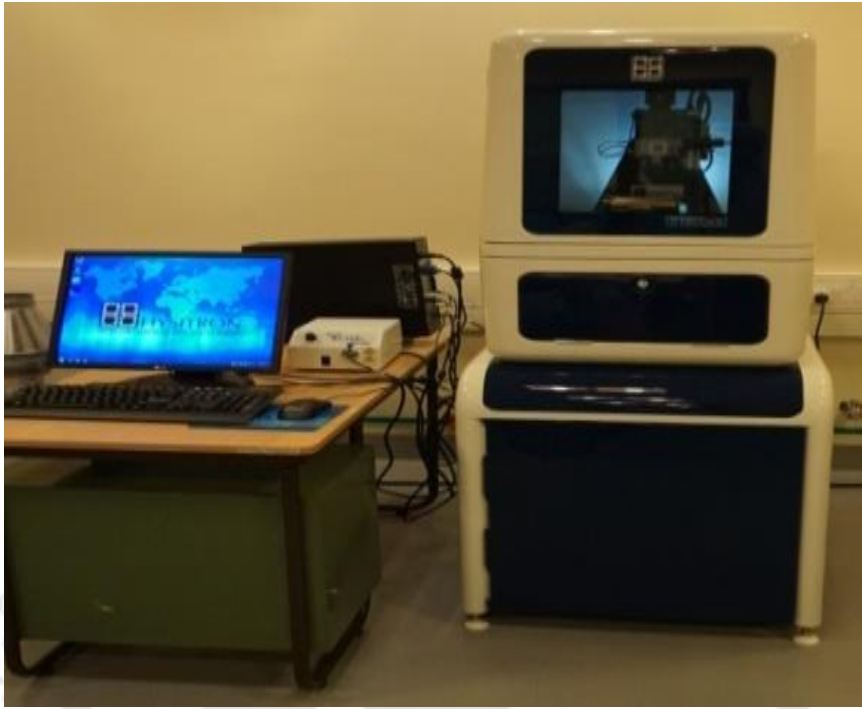
Figure 7.5: Hysitron make Ti Premier series nanoindenter
