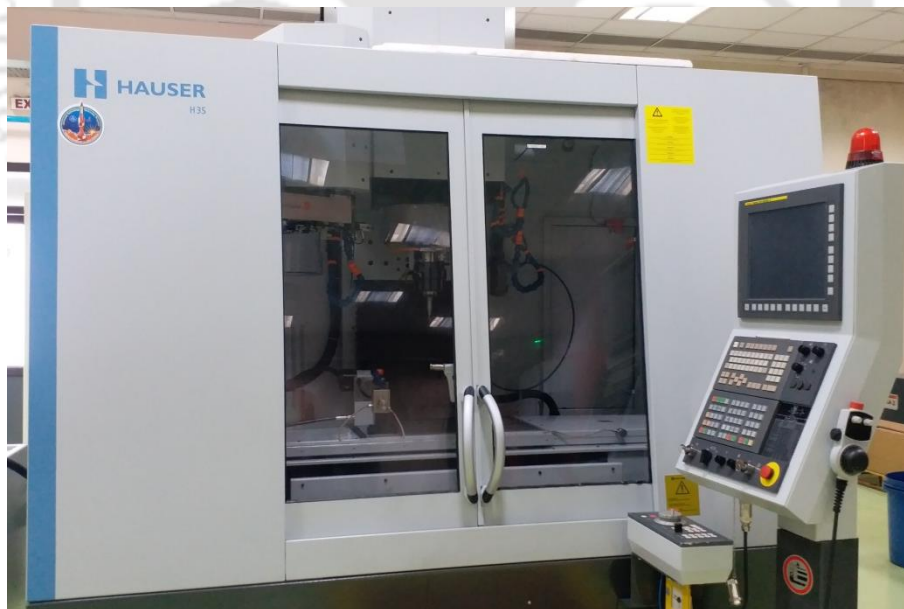
Figure 5.5: Hauser make H35 jig grinding machine for precision machining
