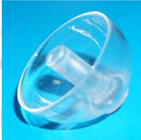
Figure 2: High precision fused silica resonator after precision machining
