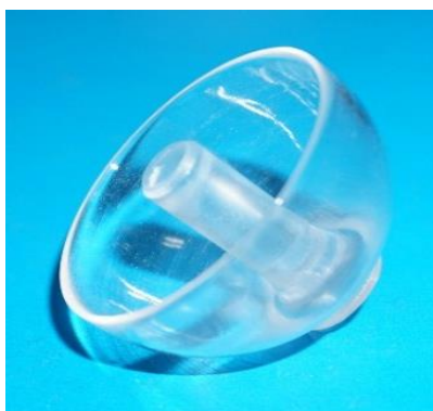
Figure 5.6: High precision fused silica resonator after precision machining
