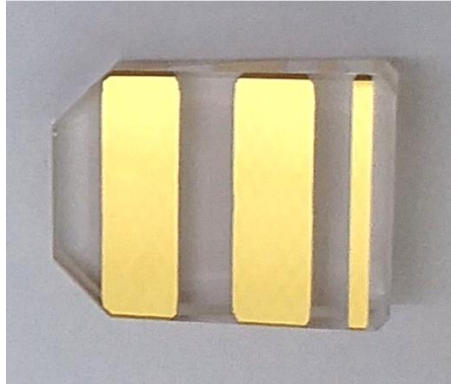
Figure 8.22: Ion beam sputtering based ultra-thin film gold coated coupon shows coated and uncoated area
