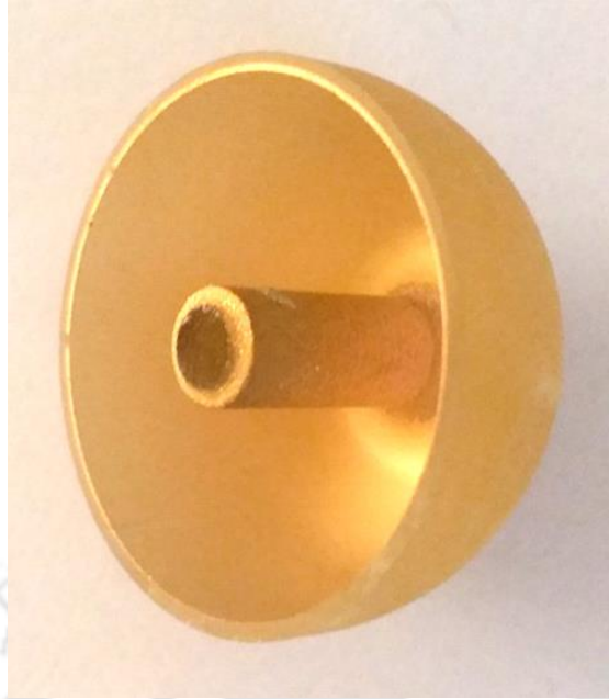
Figure 8.5: Fully gold coated fused silica resonator
