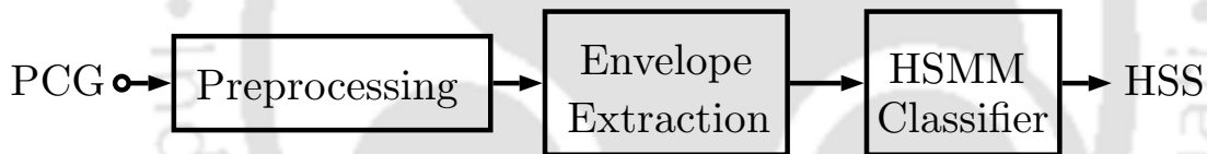
Figure 4.6: Block diagram of evaluation process with modules involved in heart sound segmentation (HSS).
