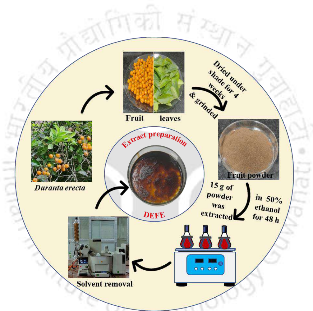
Fig. 2.4 Schematic diagram for the preparation of DEFE.
