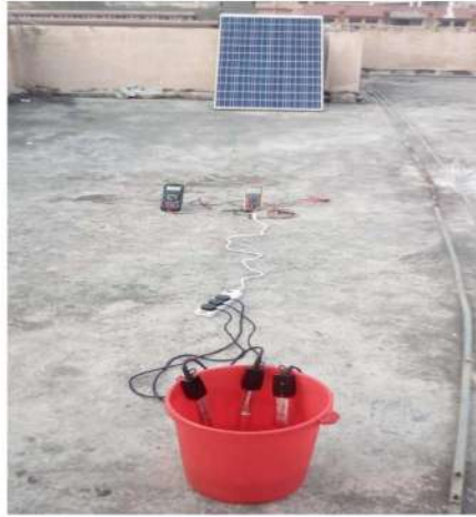
Figure 4.11: Experimental setup of PV module connected to resistive load, R = 14.0383 \Omega
