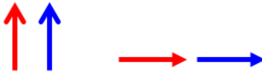
Figure 2.10: Schematic drawing of broadside and head-to-tail configurations for a pair of ferromagnetically coupled magnetic moments.
