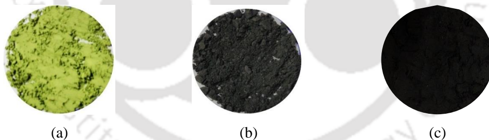
Figure 4.03: Photo view of the change in the color of the (a) pure un-milled NiO, (b) milled NiO powder for 30 hrs, and (c) milled NiO-Al powders.
