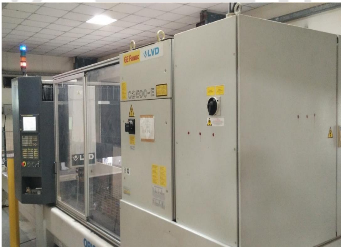
Figure 3.3 Orion 3015 2.5 kW CO 2 laser machine
