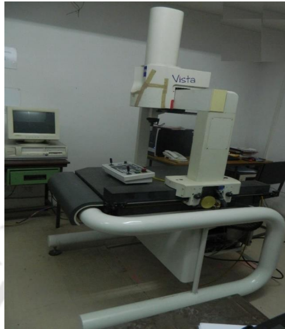
Figure 3.6 CMM machine (Make: Zeiss™; model: Vista)
