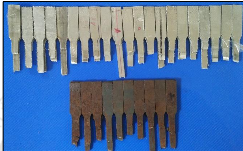
Figure 3.10 Tensile test samples after testing
