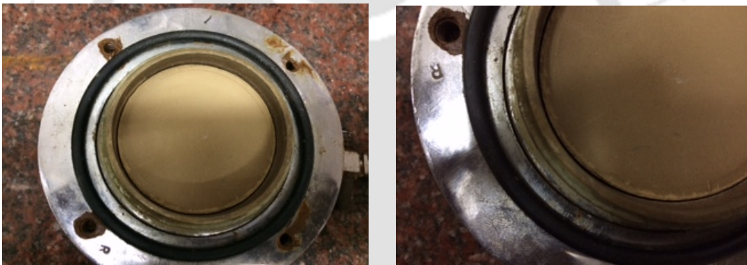
Fig. 5.3 Representation of a tiny gap created after heating of compacted bentonite
