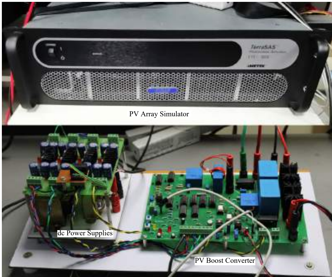
Fig. A.8 Experimental setup for PV system.
