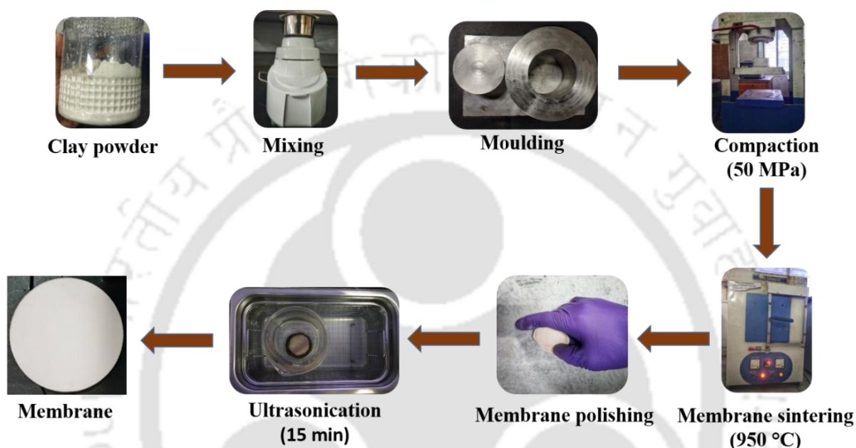
Fig. 5.1 Schematic showing membrane fabrication steps followed in this study.
