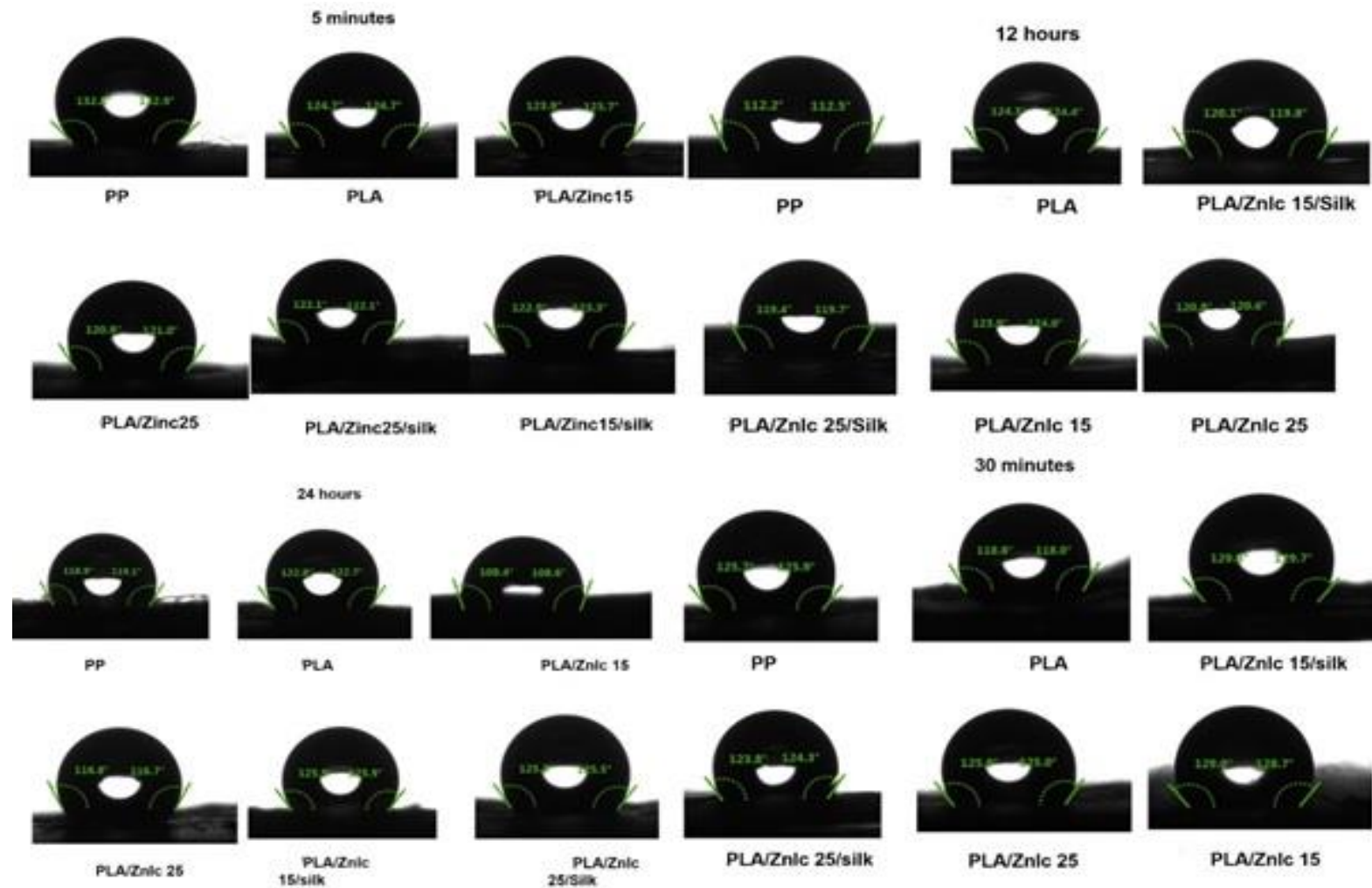
Figure 41: Water contact angle images after 5 min-24 hours of dipping treatment. This indicates reusability of the facemasks prepared.
