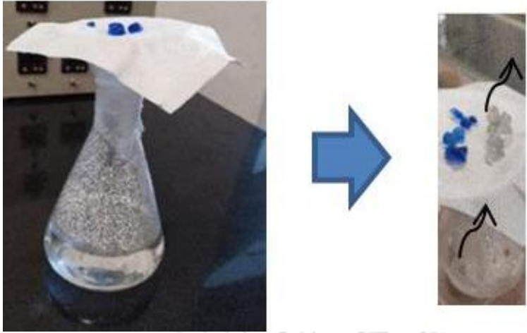
Figure 39: Silica gel placed over nanofabric changed its color from blue to pink signifying its breathability.
