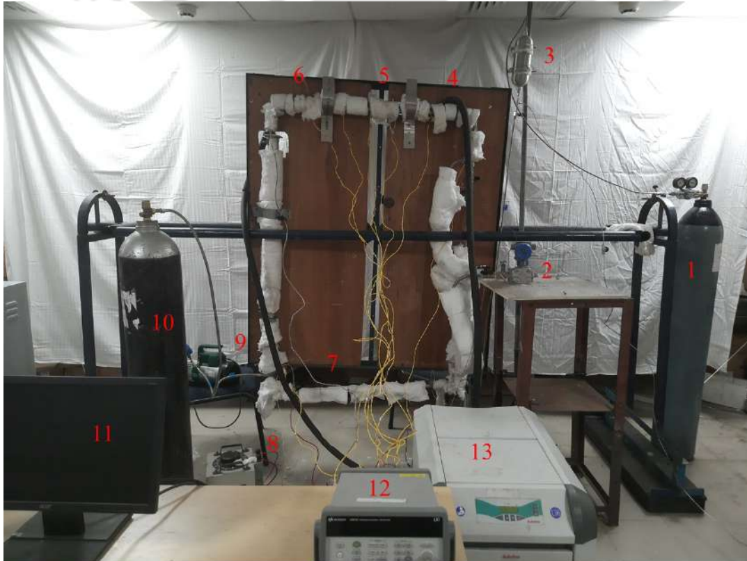
1. N 2 cylinder 2. DPT 3. Pressurizer 4. Water inlet 5. Cooler 6. Water outlet 7. Heater 8. Variac 9. Vacuum pump 10. CO 2 Cylinder 11. Computer 12. DAS 13. Chiller
