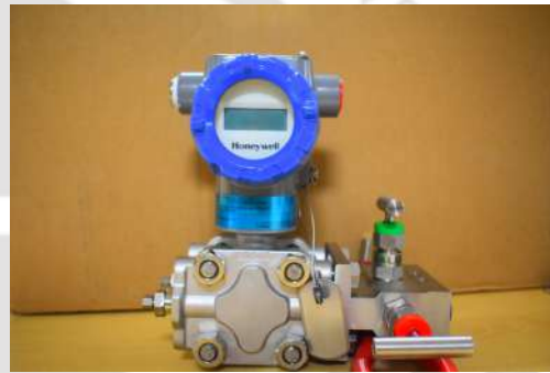
(b) Honeywell make differential pressure transmitter
