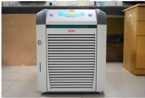
(a) Julabo make recirculating chiller
