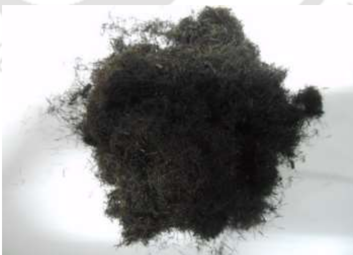
Figure 2.2b: PANI coated jute polymer
