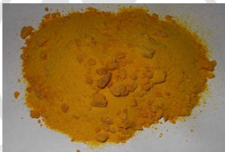
Figure 2.1c: AFC coated silica gel
