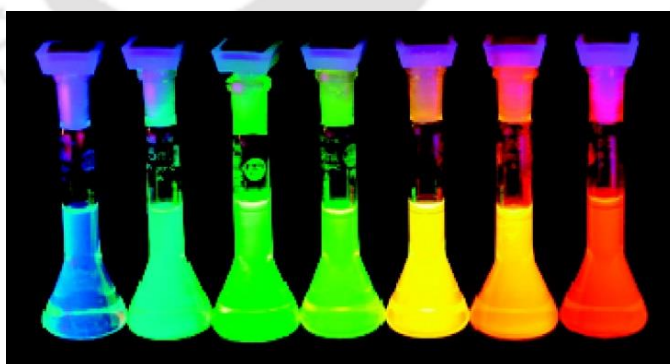
Figure 1.2. Fluorescence image of 1.7 to 5 nm sized CdSe/ZnS core-shell Qdots. (Reprinted with permission from reference 19. Copyright 2002 John Wiley and Sons)
