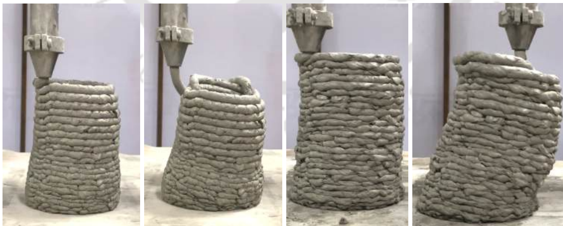
(h) C10F10P2 (failed at 24 th layer)
