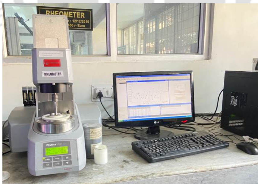
Figure 4.4: Rheometer with concentric cylinder geometry to measure viscosity of surfactant.
