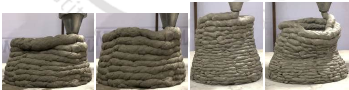
(b) C10P2 (failed at 10 th layer)
