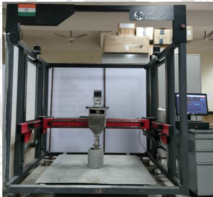
Figure 4.3: 3D concrete printer setup (Panda and Tran 2022; Dey et al., 2023).
