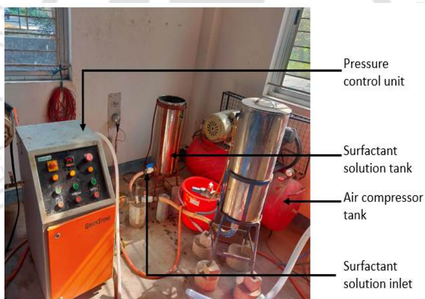
Figure 4.2: Foam generator set up
