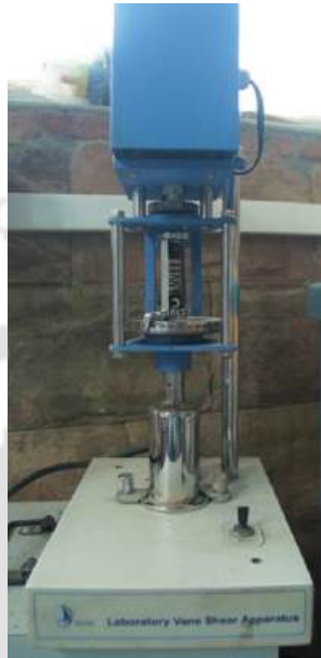
Figure 4.8: Laboratory vane shear test set up.
