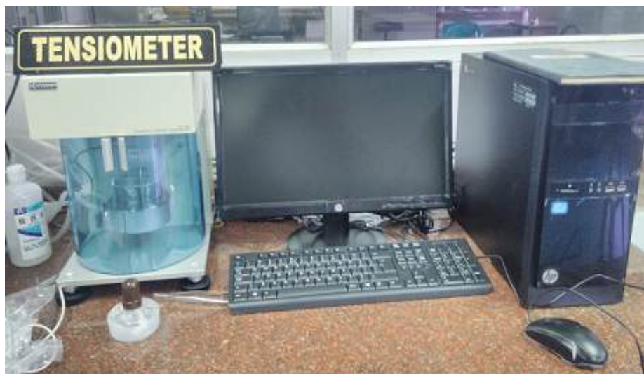
Figure 4.5: Tensiometer for measuring the surface tension of the surfactant.
