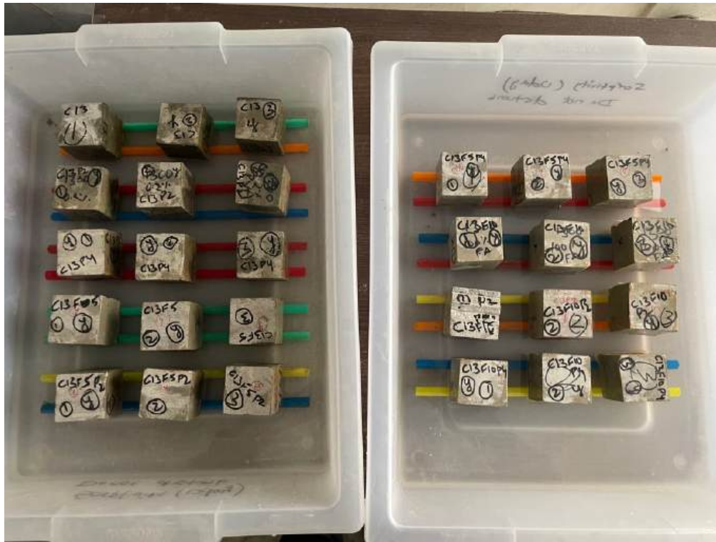
Figure 5.9: Sorptivity measurement of 3DP-FC samples
