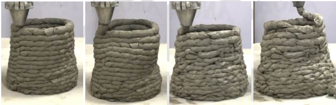
(f) C10F5P2 (failed at 18 th layer)
