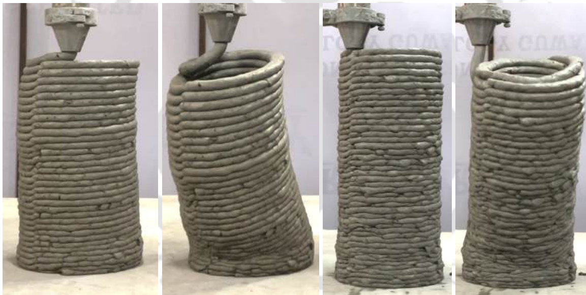
(f) C13F5P2 (failed at 35 th layer)
