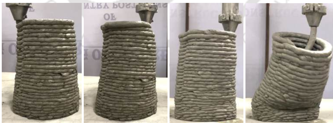
(b) C13P2 (failed at 30 th layer)
