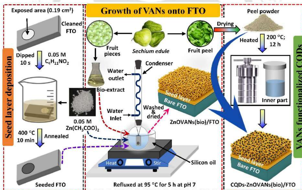
Figure 2.7: Schematic steps depicting 2D ZnO VANs synthesis onto FTO glass and its functionalization with CQDs.
