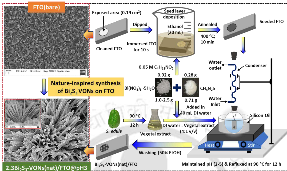
Figure 2.8: Schematic illustration of the nature-inspired synthesis protocol for the formation of \text{Bi}_2\text{S}_3 VONs on the FTO glass substrate.
