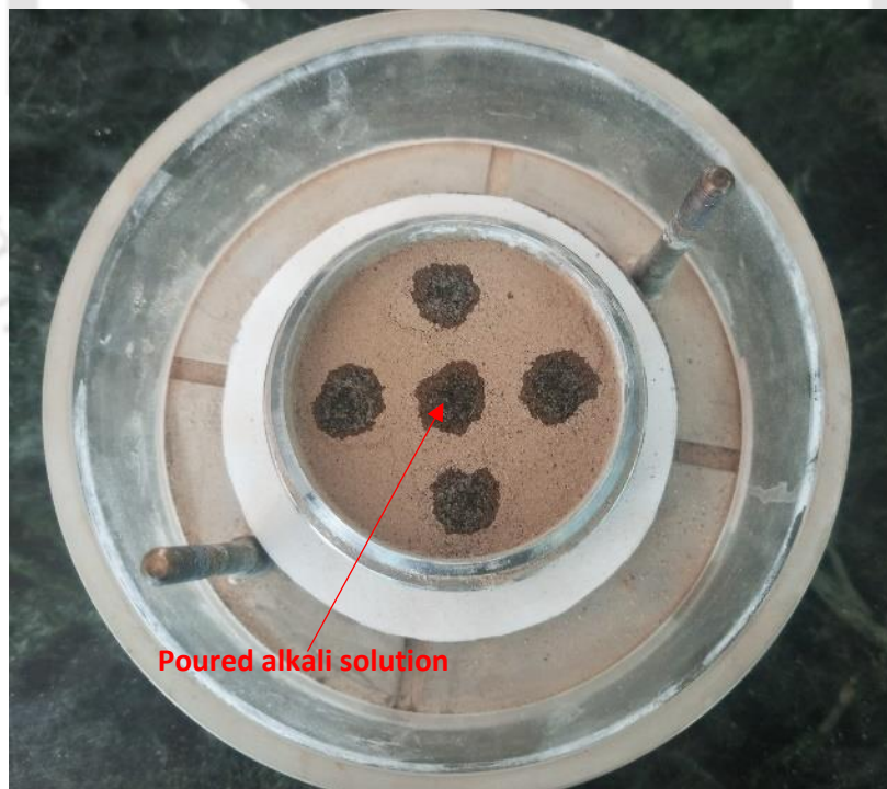
Fig. 3.18. Kaolin samples compacted in pattern A inside the oedometer ring: Moment just after the application of alkali activator solution.
