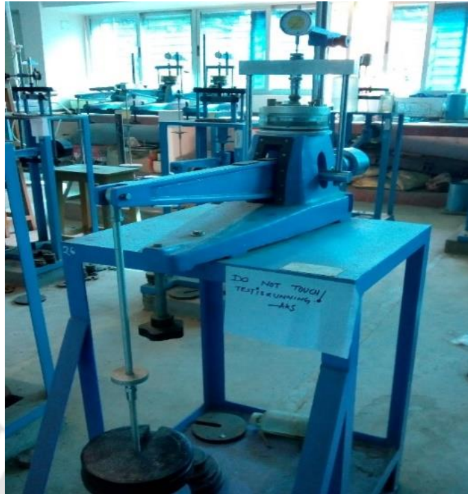
Fig. 3.8. Laboratory oedometer set-up.
