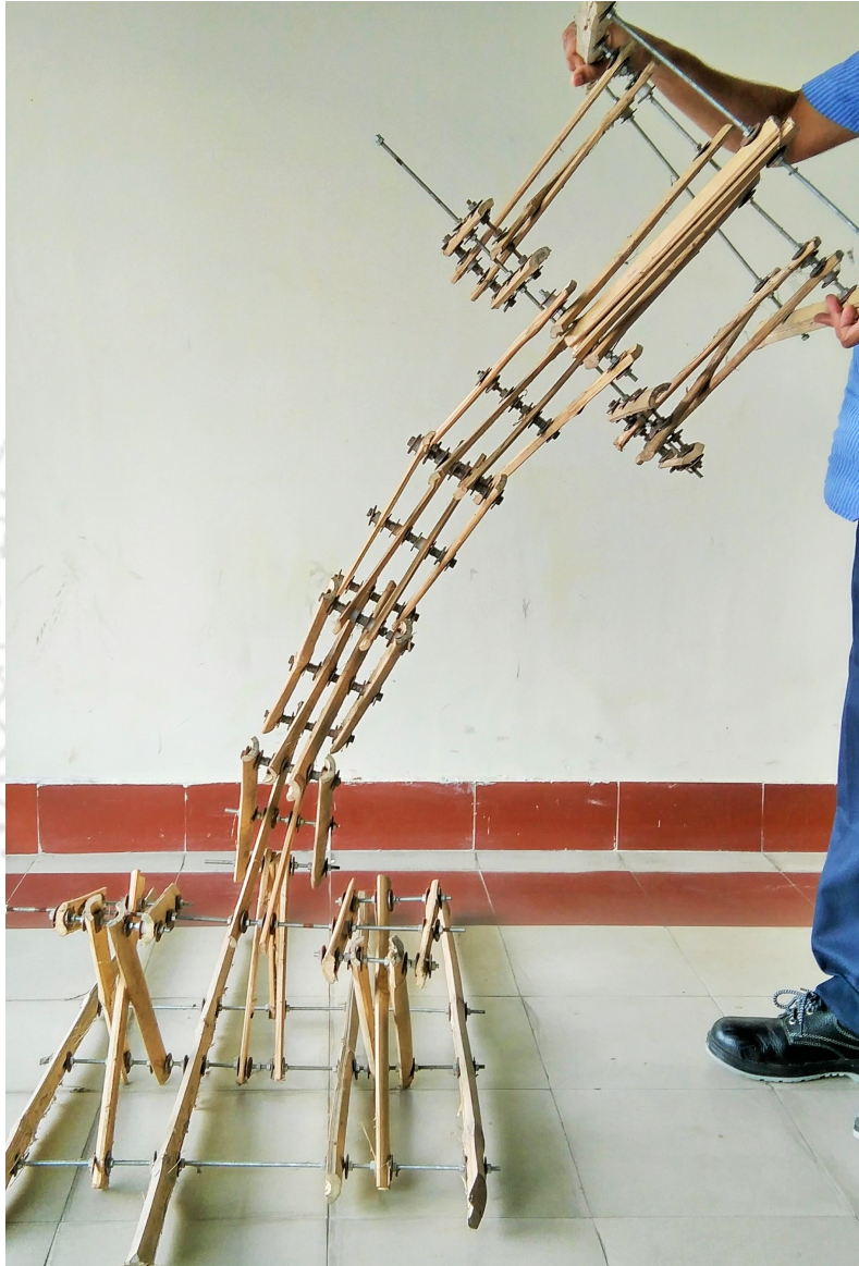
Figure 1.3: Lateral sway in the fabricated parallel-plane scissor linkage.
