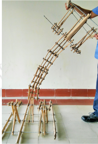
Figure 3.3: Lateral sway in parallel-plane scissor linkage.
