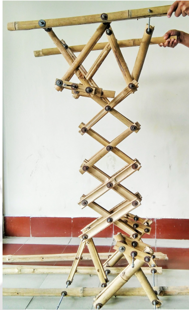
Figure 3.2: Parallel-plane scissor linkage made by bamboo strips.
