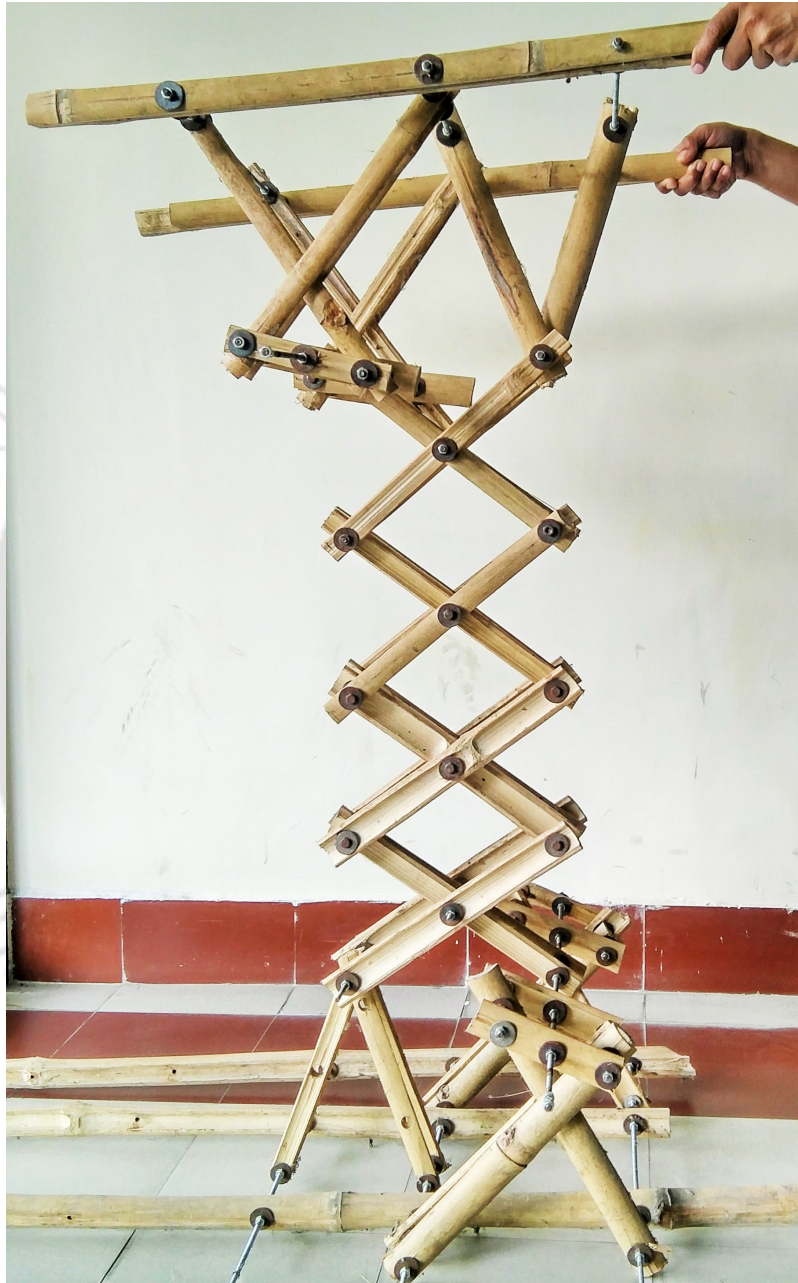
Figure 1.2: Fabricated parallel-plane scissor mechanism.
