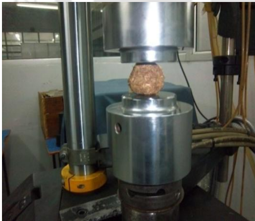
Fig.3.15 Compression test of briquette
