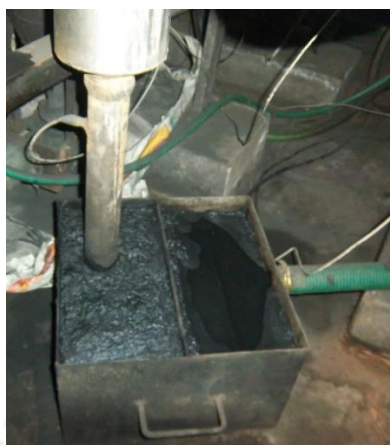
Fig. 1 Tar collected in water tub
