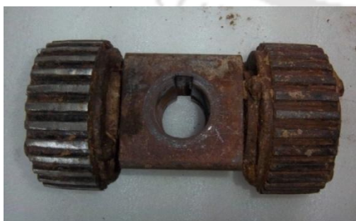
Fig. 4.30 Rollers of the Pellet press.
