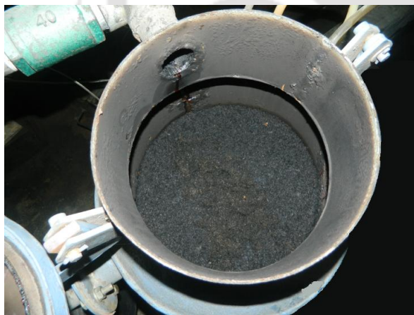
Fig. 3 Tar deposited in coarse filter
