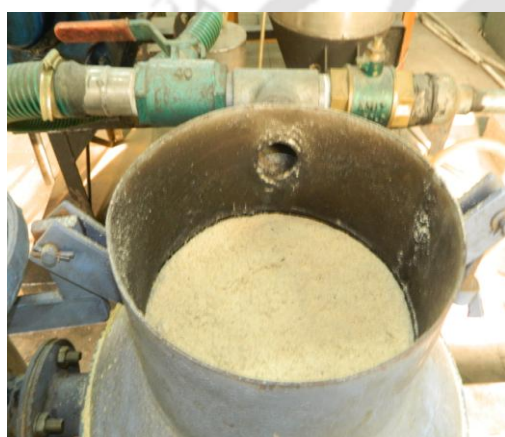
Fig.4.7 (a) Coarse filter with saw dust as filter material. Fig. 4.7(b) Fine filter with fabric material bag as filter.
