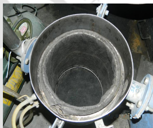
Fig.4.7 (a) Coarse filter with saw dust as filter material. Fig. 4.7(b) Fine filter with fabric material bag as filter.
