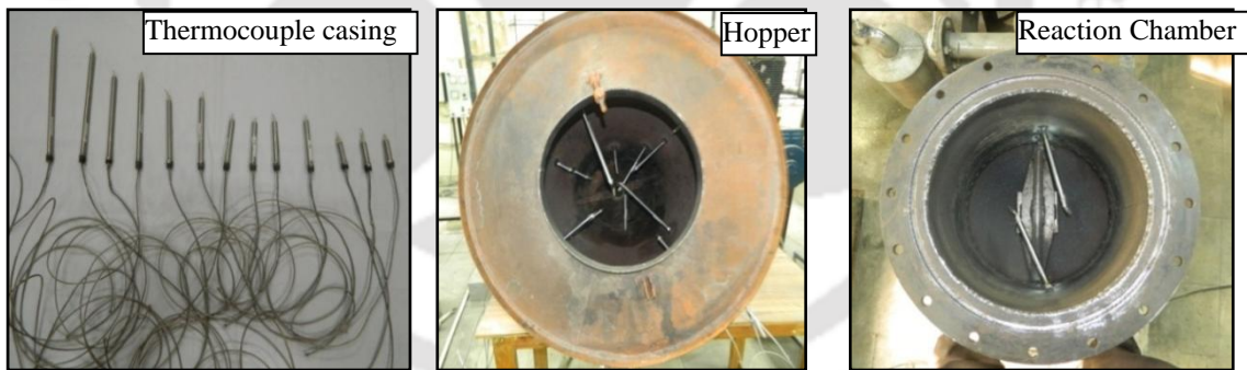
Fig. 4.10(c) Reaction chamber with thermocouple casings
