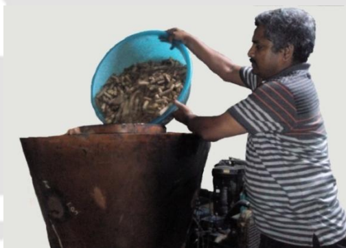
Fig. 4.18 Feeding of gasifier
