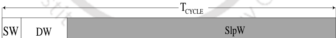
Figure 1.1: Cycle structure followed by the network nodes in generic contention based synchronous MAC protocols.
