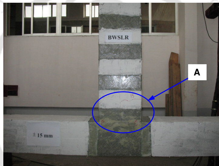
Fig. 6.4 Appearance of first rupture in BWSLR specimen at \pm 15 mm amplitude
