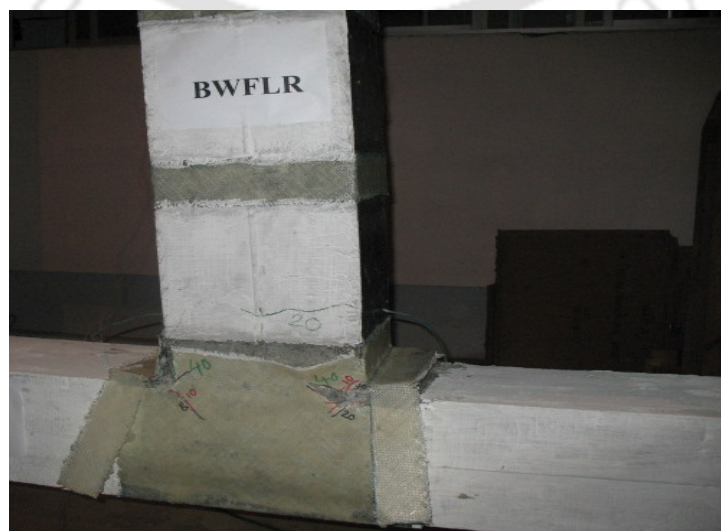
Fig. 5.7 BWFLR specimen at the end of test
