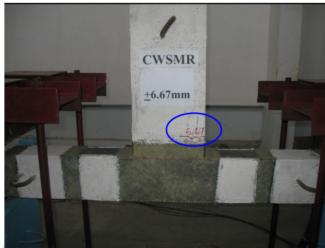
Fig. 7.15 Appearance of first visible crack in CWSMR specimen
