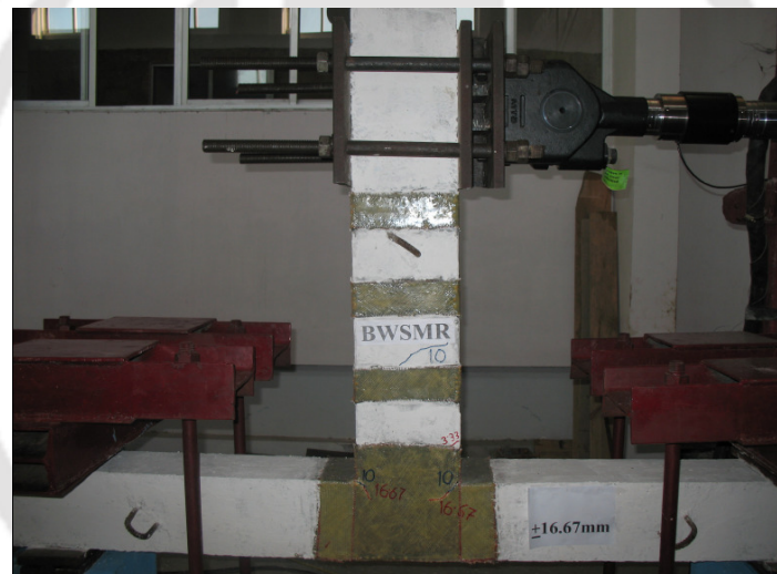
Fig. 6.14 Appearance of rupture in GFRP of BWSMR specimen
