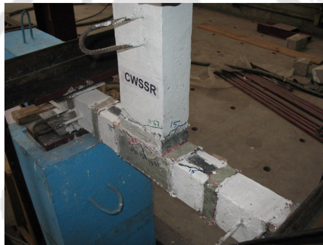
Fig. 7.26 CWSSR specimen at the end of testing
