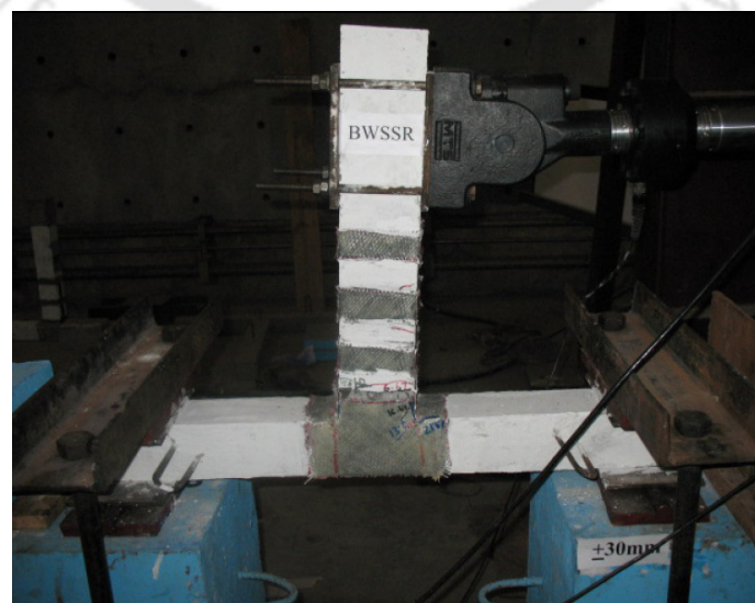
Fig. 6.24 BWSSR specimen at the end of test
