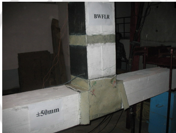
Fig. 5.6 Delimitation of FRP sheets near joint region in BWFLR specimen
