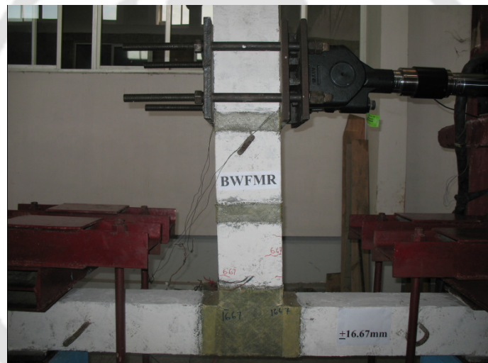
Fig. 5.17 Appearance of rupture in GFRP sheet for BWFMR specimen
