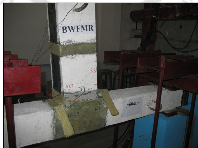
Fig. 5.18 BWFMR specimen at the end of the test
