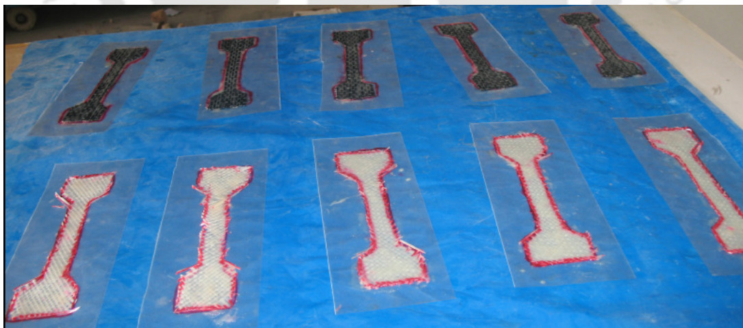
Fig. 2.2 Test coupons for CFRP and GFRP
