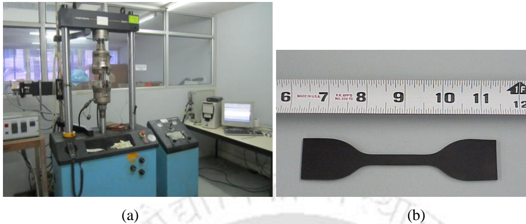
Figure 6.21 (a) tensile test setup and (b) ASTM standard specimen
