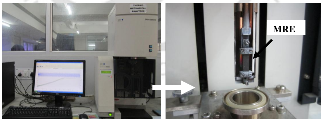
Figure 6.13 Photograph of DMA/TMA instrument with metallic probe.
