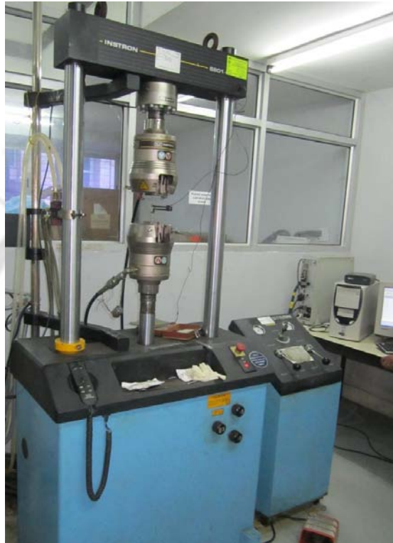
Figure 6.23 Photograph of an universal testing machine (INSTRON-8801, 100 kN capacity) for tensile test of aluminum and MRE.
