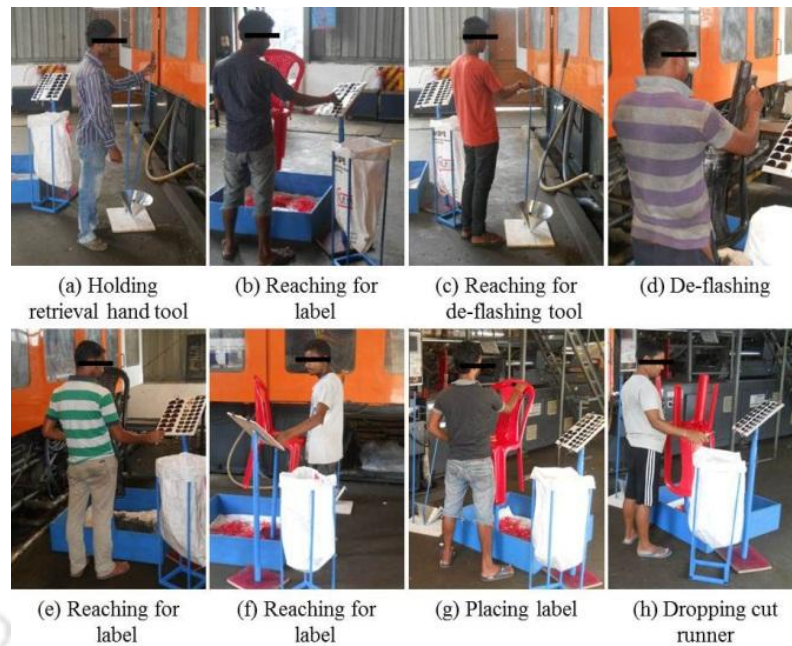
Figure 4.22 Trials by different workers in proposed model of the injection-molding workstation fixtures
