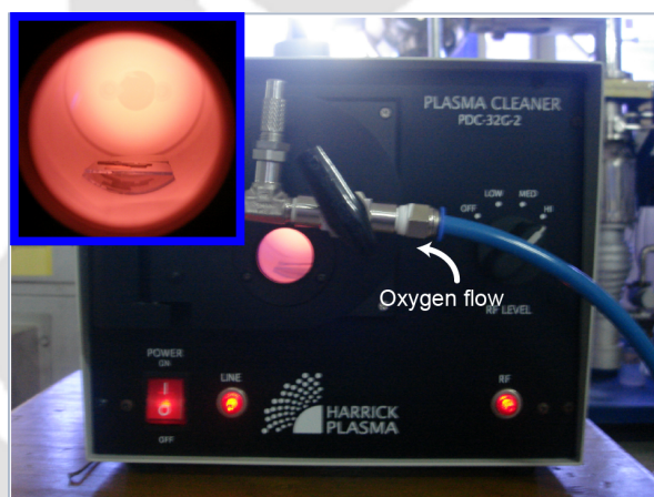
Figure 2.2: Photograph of the plasma cleaner (HARRICK PLASMA, PDC-32G-2, U.S.A) used for the removal of the bottom graphene deposited on the backside of the Cu foil in the CVD growth. Inset shows the exposure of oxygen plasma on graphene samples.
