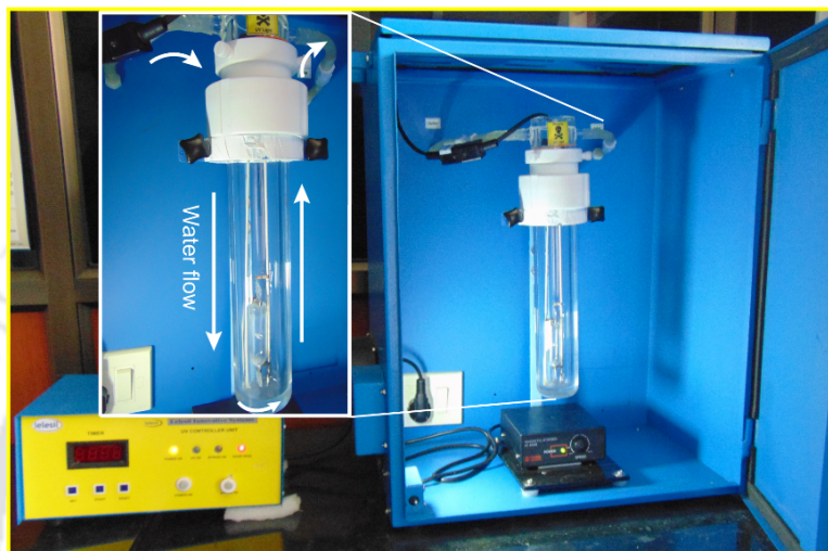
Figure 2.17: Photograph of visible Photocatalysis setup, which consists of a Xenon Lamp, Power-250 Watt with a wavelength range from 400-800 nm. Note that the arrows indicate the water circulation during the irradiation of sample in-order to reduce the heating effect on the photocatalysts.
