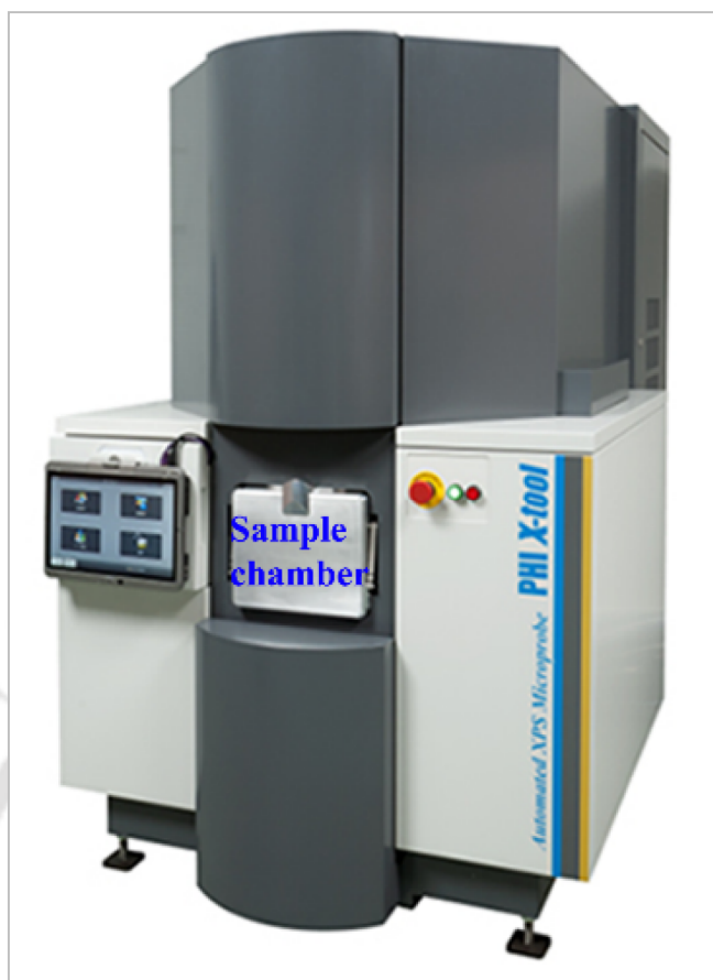
Figure 2.13: Photograph of the XPS spectrometer (PHI-Xtool, UlvacPhi) using an Al K \alpha X-ray beam (1486.7 eV).
