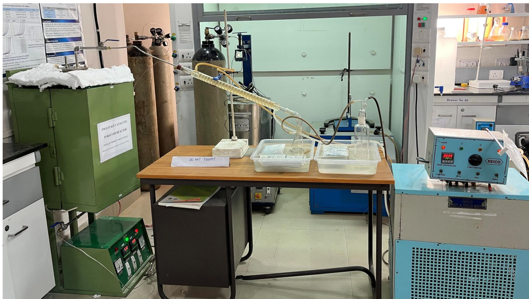
Fig 2.10. Experimental setup for catalytic pyrolysis reactor assembly, with ondenser, and circulating chiller used for semi-batch catalytic pyrolysis experiments.
