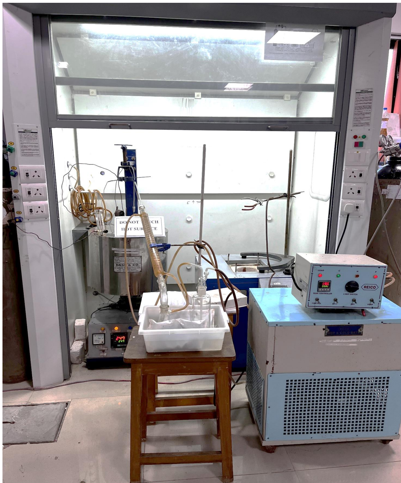
Fig 2.8. Experimental setup for pyrolysis reactor assembly, with condenser, and circulating chiller used for standard pyrolysis and co-pyrolysis experiments at atmospheric pressure.
