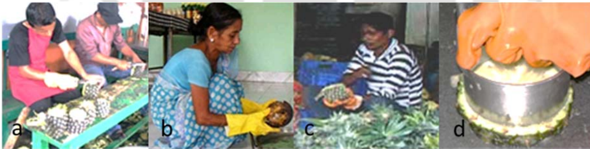
Figure 3.04 Techniques, tools used for pineapple peeling task; a- Peeling the pineapple supporting it on a base, b - Peeling using Baithi , c- Peeling using knife by holding pineapple in one hand, d- others like using punch cutter
