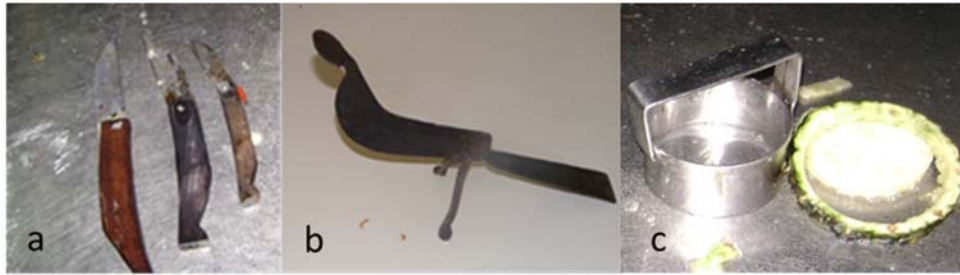
Figure 3.05 Different peeling tools: a- variety of knives, b- Baithi, c- punch cutter
