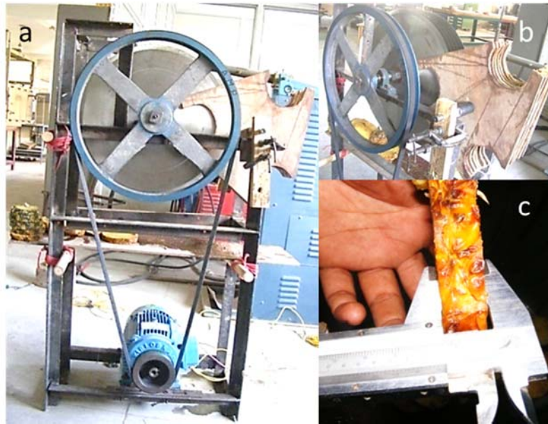
Figure 4. 35 Proof of concept of the slicing Machine; a- Assembly, b- Working, c- Output
