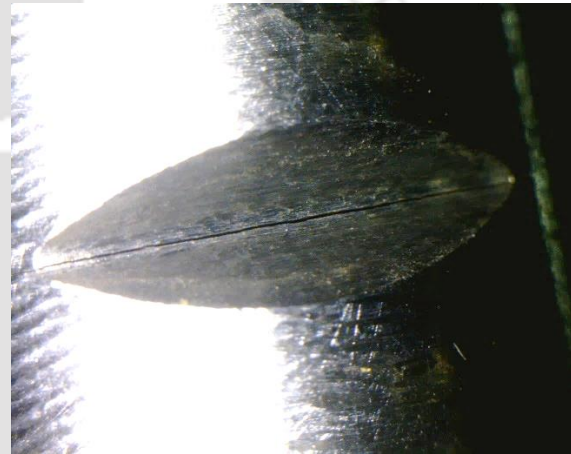
Figure 3.6 Close view of the fatigue crack at tip of a notch on the shaft
