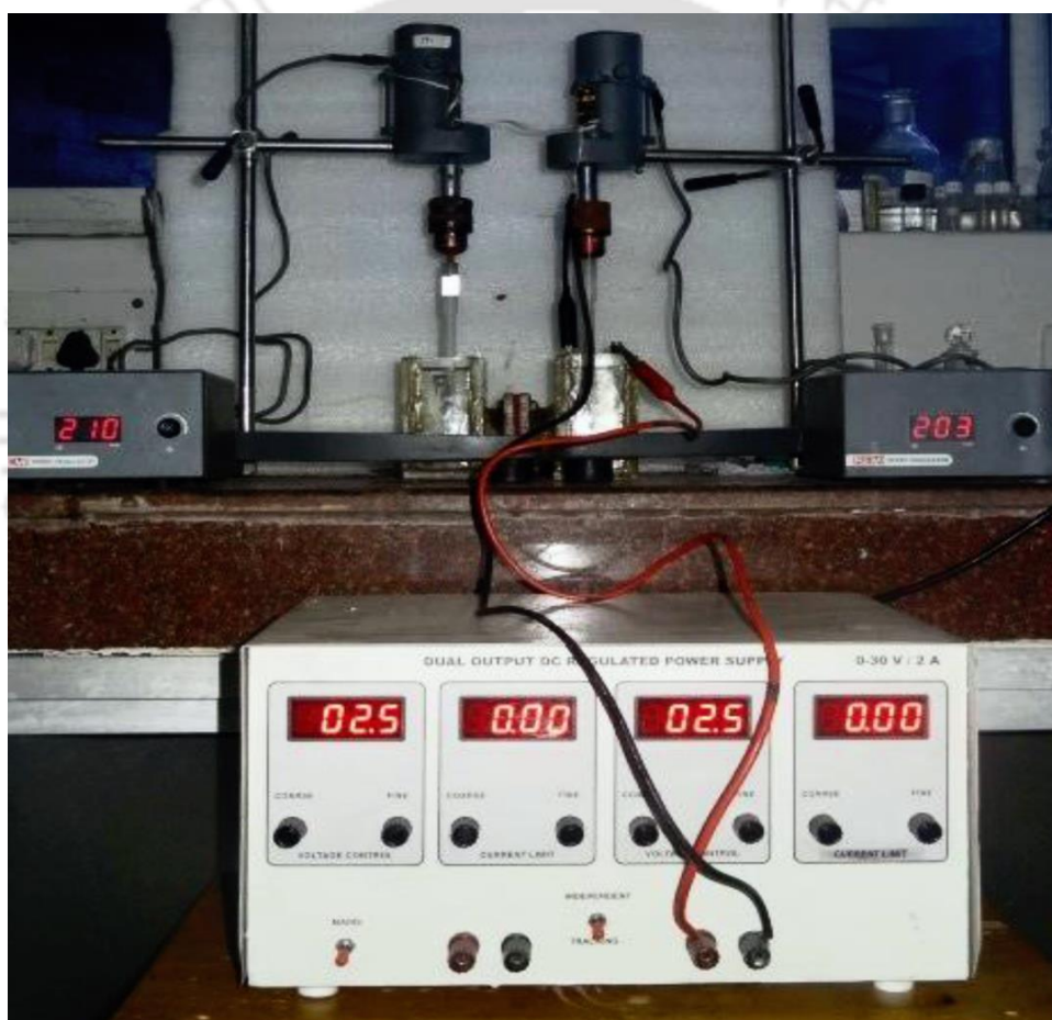
Figure 2.5: Photograph of FS-SLM with electro-deposition experimental set-up
