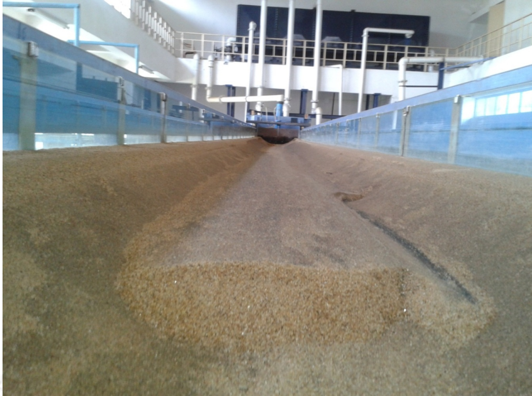
Figure 2.24: Channel cross section at the end of seepage experiment on coarse sand of median diameter = 1.1 mm
