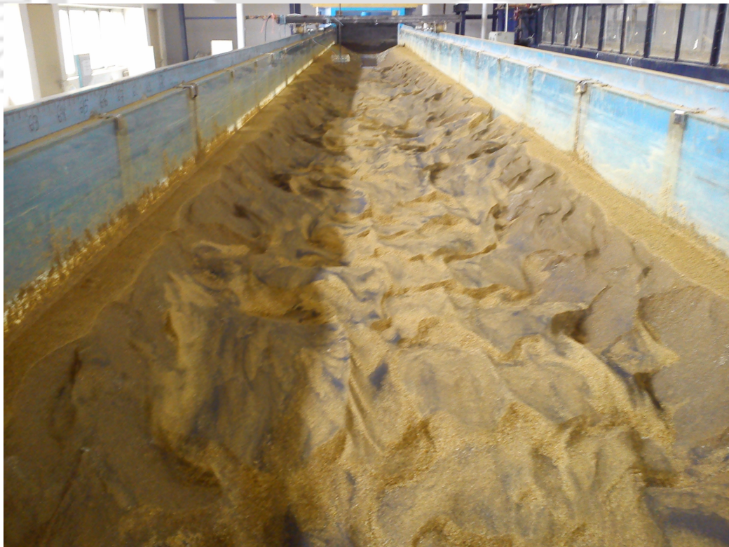
Figure 4.17: Snapshot of channel bed at the end of 15% seepage experiment
