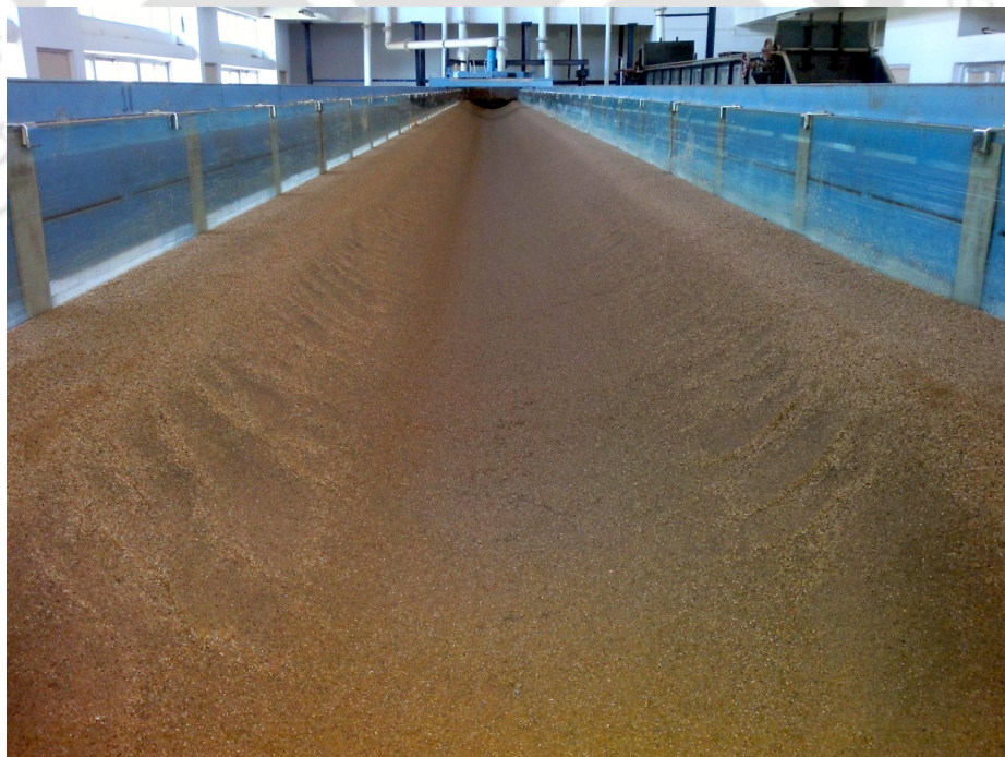
Figure 2.20: Channel after successful completion of no seepage experiment
