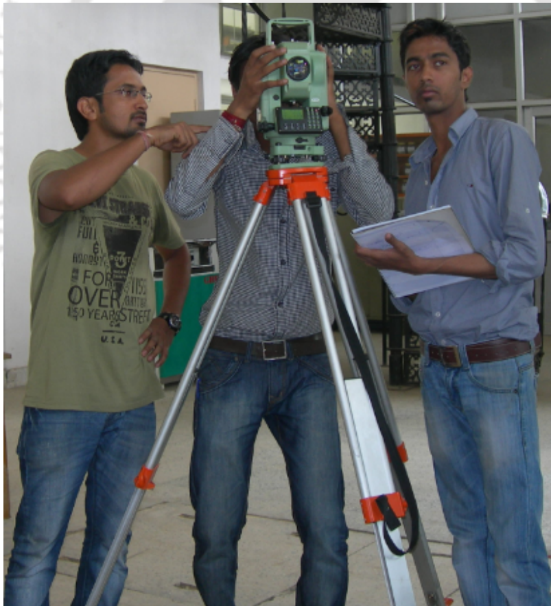
Figure 2.11: Snapshot of the total station to measure the slope of channel bed
