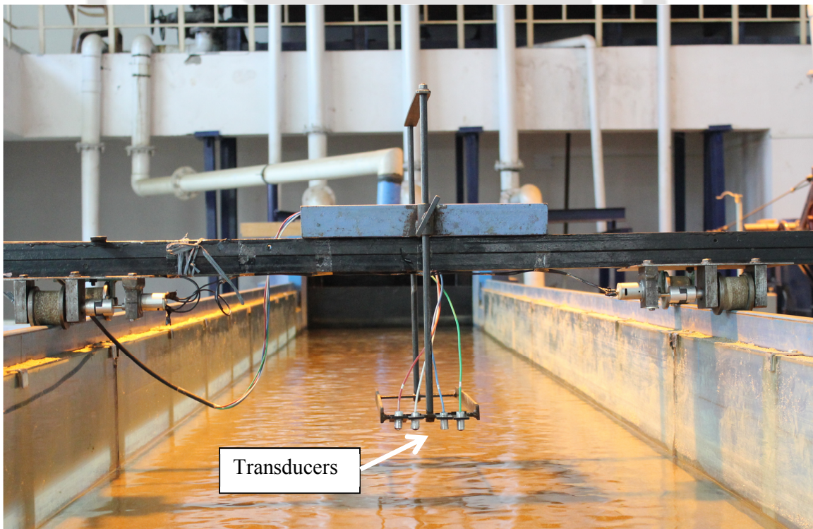
Figure 2.12: Transducers of SeaTek Ultrasonic Ranging System with automated moving trolley
