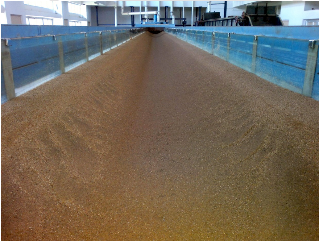
Figure 4.16: Snapshot of channel bed after no seepage experiment
