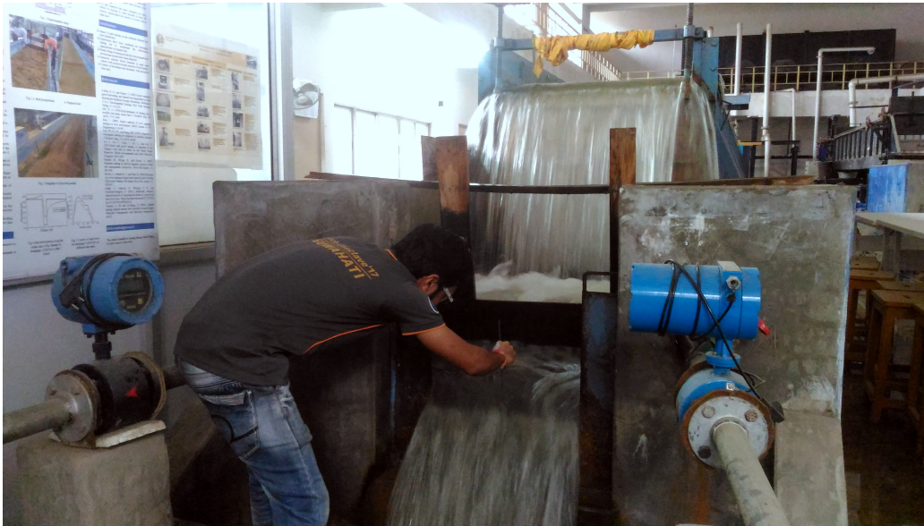
Figure 2.6: Measurement of main channel discharge over rectangular notch located at downstream end of the flume
