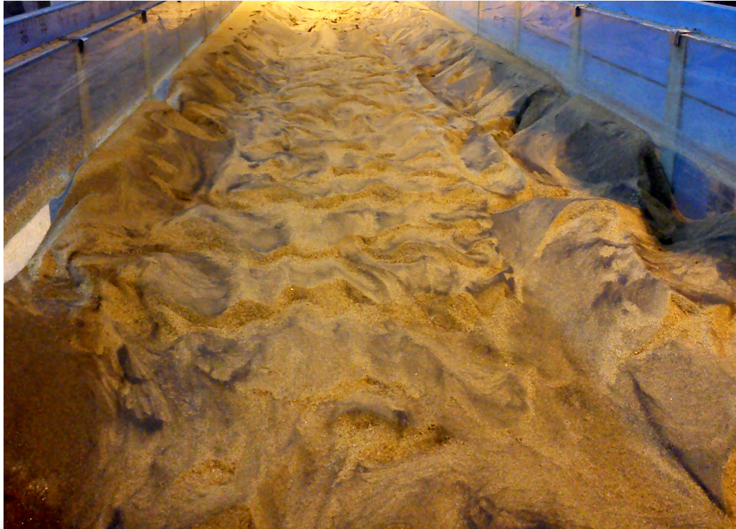
Figure 2.23: At the end of seepage experiment after 31 h of run
