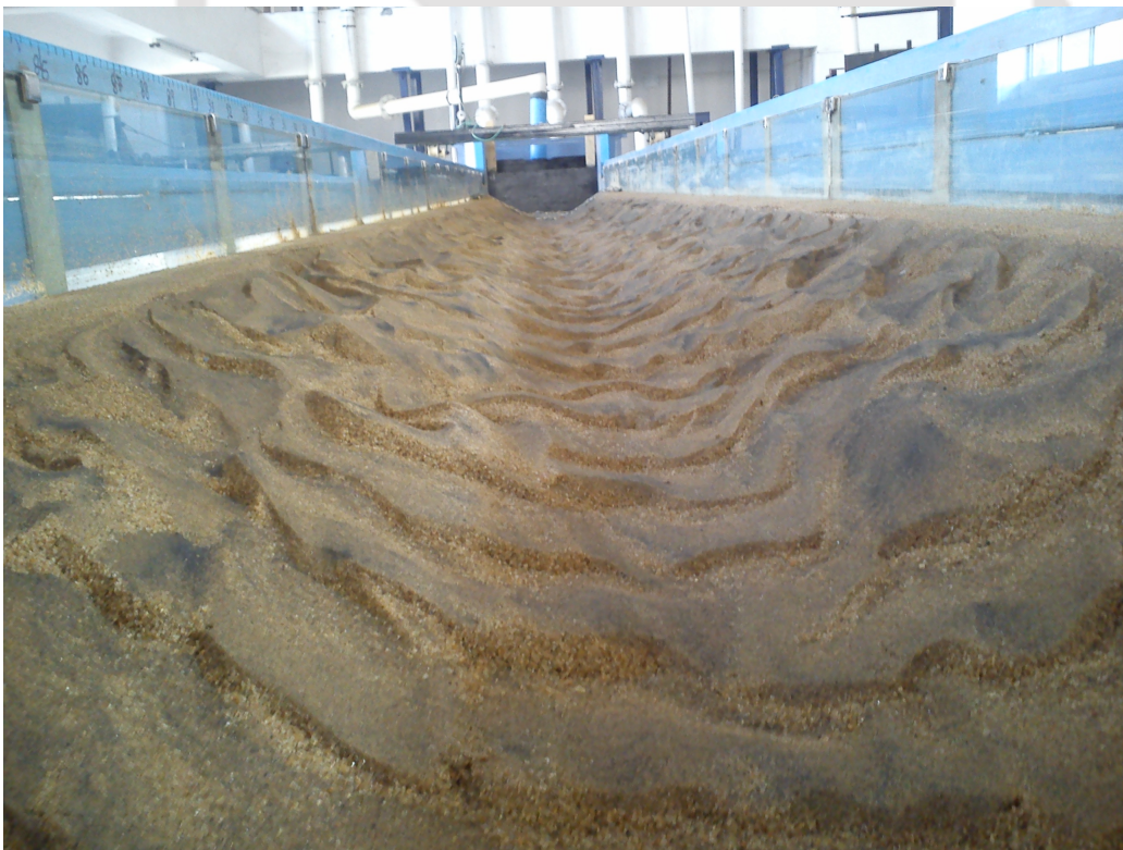
Figure 2.22: Snapshot of the channel during run after 3 h run with the application of downward seepage on the sand of D_{50} = 0.41 mm
