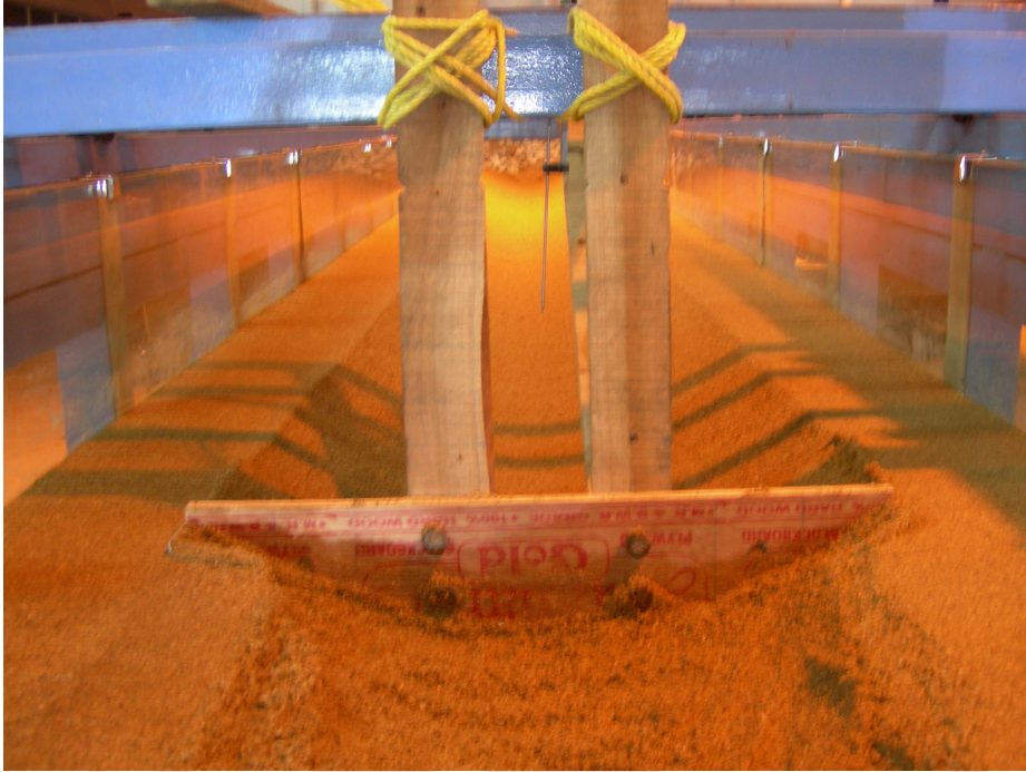
Figure 2.18: Wooden shaper for preparing the Lane's (1953) geometric profile in the flume
