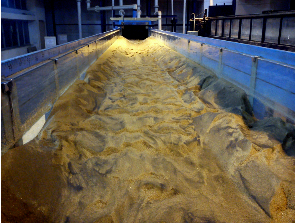
Figure 4.18: Snapshot of channel bed at the end of 20% seepage experiment
